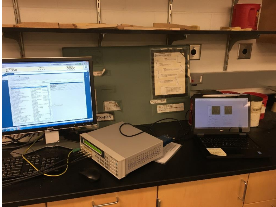
Figure 28: Data acquisition system and laptop used to record the readings
