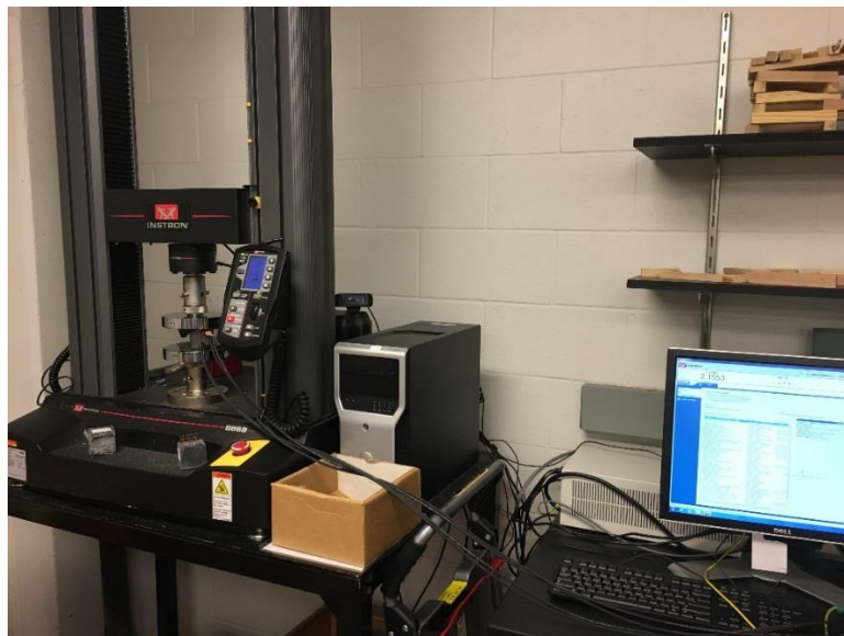
Figure 27: Instron machine used to apply a strain controlled loading on the samples
