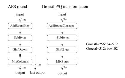
Figure 2.8: Block diagram of Grøsl and AES round
