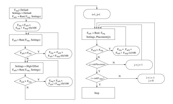
Figure 6.4: ATHENa GMU\_optimzation\_1 method for Xilinx devices
