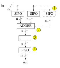
Figure 3.6: Test circuit for addition and modular addition
