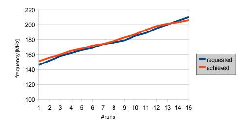
Figure 6.3: Dependency between requested and achieved frequency for combined optimization targets
