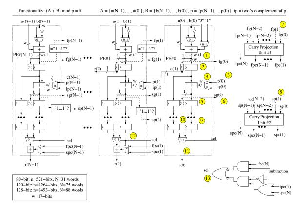
Figure 4.2: Pipelined high-radix carry save modular adder/subtractor
