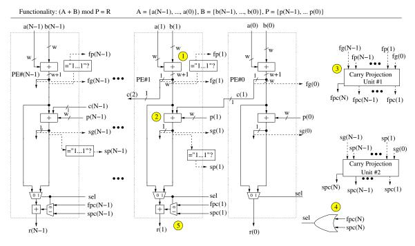
Figure 3.5: Modular adder based on the hybrid adder
