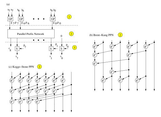
Figure 3.1: (a) General concept of the parallel prefix addition, (b) Brent-Kung adder, (c) Kogge-Stone adder. GP:  $g_i = x_i \cdot y_i$ ,  $p_i = x_i \oplus y_i$ , S:  $s_i = p_i \oplus c_i$ ,  $\emptyset: g = g'' + g' \cdot p'', p = p' \cdot p''$
