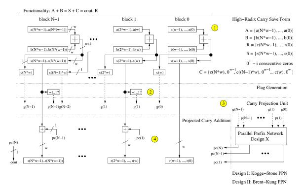
Figure 3.2: Hybrid radix- $2^w$  carry save adder with the carry projection unit based on parallel prefix network (PPN). Design X - Design I is based on Kogge-Stone PPN and Design II is based on Brent-Kung PPN
