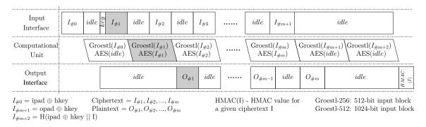
Figure 2.15: High level scheduling in the Grøstl/AES core during decryption process
