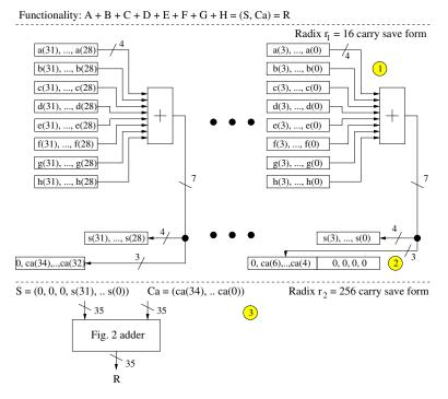
Figure 4.3: High-radix carry save multi-operand adder
