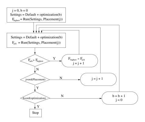
Figure 6.5: ATHENa GMU\_optimzation\_1 method for Altera devices
