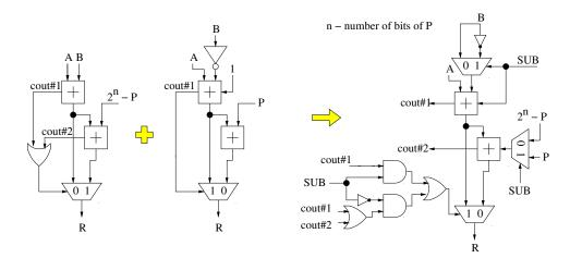
Figure 4.1: Modular adder/subtractor - high level block diagram
