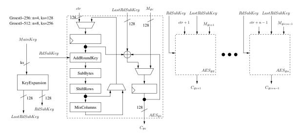
Figure 2.12: Block diagram of AES-CTR where n is the number of AES cores
