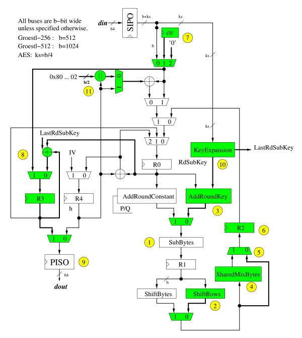
Figure 2.10: Block diagram of Grøstl/AES core
