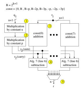
Figure 4.6: Block diagram of Barrett reduction for Solinas primes
