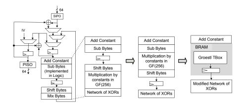
Figure 2.2: Phases in the Grøstl-0 round transformation to T-box representation.
