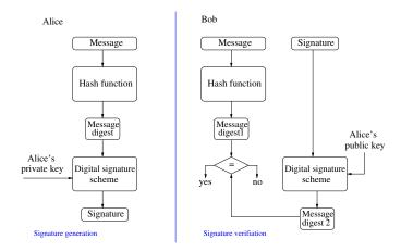
Figure 1.1: Digital signature generation and verification
