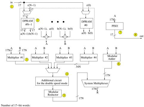
$\begin{aligned} &\text{Number of } 17\text{-bit words.} \\ &\text{N} = 31 \ (80\text{-bit}), \ 75 \ (120\text{-bit}), \ 88 \ (128\text{-bit}) \\ &\text{A} = \{a(N\text{-}1), \dots a(0)\}, \ B = \{b(N\text{-}1), \dots b(0)\}, \ R = \{r(N\text{-}1), \dots r(0)\} \end{aligned}$
