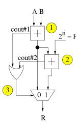
Figure 3.4: Modular adder based introduced in [20]
