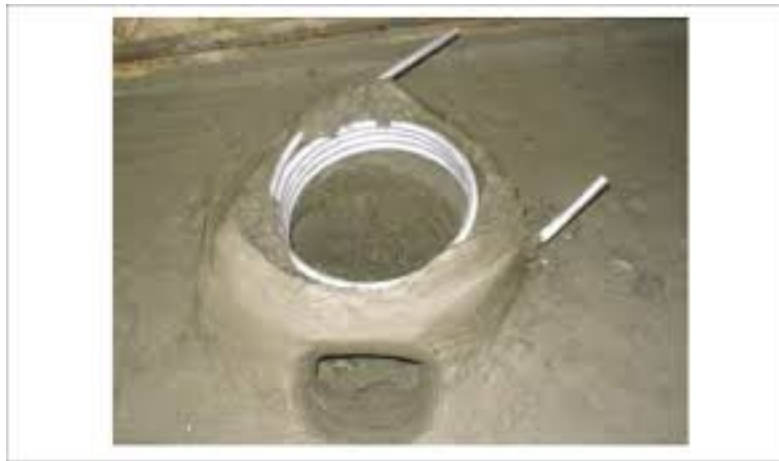
Figure 9: Inside view of the chulli system showing the aluminum coil water flows through (reprinted with permission of JSTOR) (Islam et. al., 2006)
