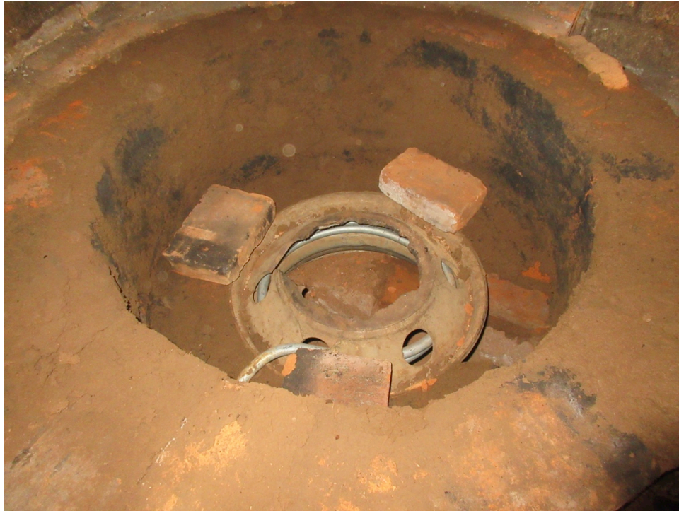
Figure 29: A close-up look inside the stove from Figure 28 highlighting the location of the coiled pipe. After flowing through the hosepipe explained in Figure 28, water passes through this coil where it is heated. After heating in the coil, water flows out of the effluent tap also shown in Figure 28.
