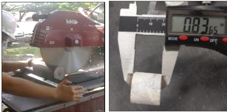
Figure 5.1 (a) Cut concrete cylinders (b) sample dimension
