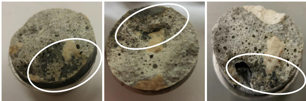
Low Porosity -Dark circled area shows epoxy penetration, More pores visible
