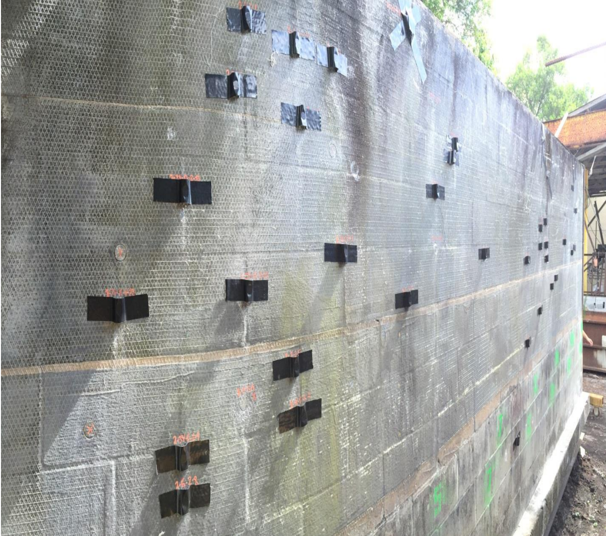
Figure 9.12 Dolly layout out in wall 3 (tonen). On CFRP surface, over bed, head and intersecting joints
