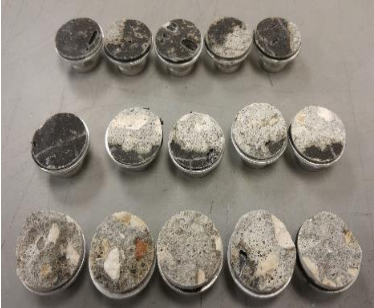
Figure 8.2 Failure mode after moisture exposure. Failure Mode: G (Concrete Substrate failure), E (FRP/concrete interface), F (mixed mode G and mode E)
