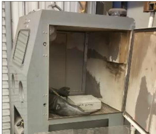
Figure 4.3 Slabs in sandblaster
