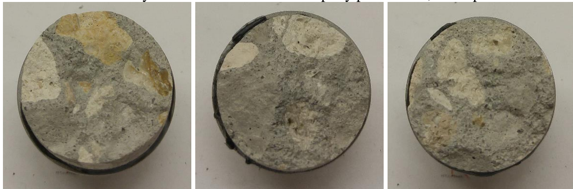
Medium Porosity – some pores visible but no epoxy Figure 8.11 Dolly plan-view from control specimens
