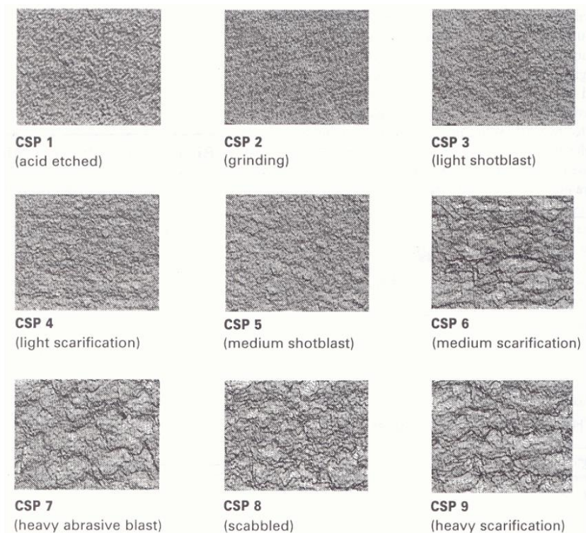
Figure 2.1 Concrete surface profiles. Reprinted from NCHRP 609, Attachment C. Permission to use from National Academy of Sciences
