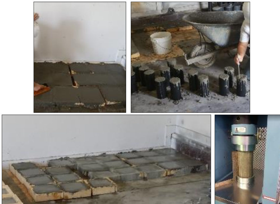
Figure 4.2 Casting, curing and testing concrete
