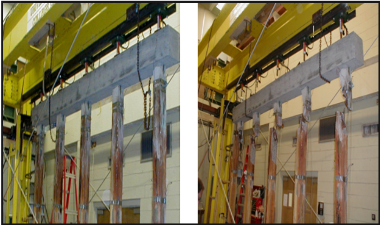
Figure 2.7 50% damage bent prior to testing.
