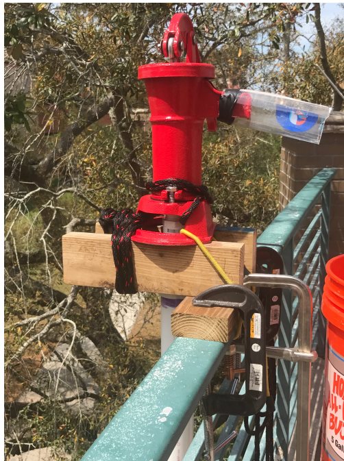
Figure 3.2: Simmons Manufacturing Pitcher Pump #1160 secured on pump stand
