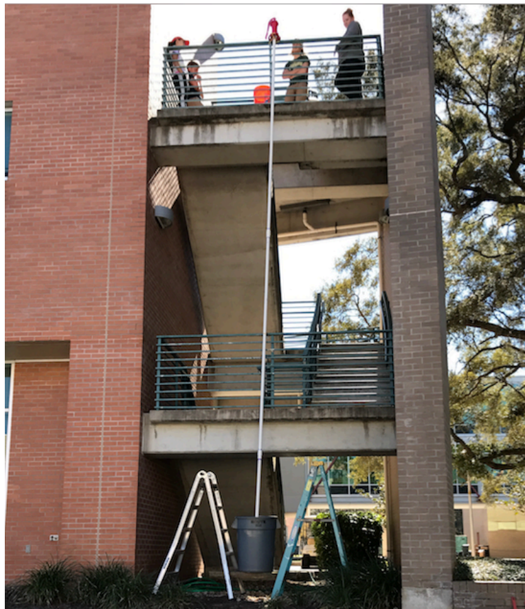
Figure 3.1: Testing set-up at seven meters using 1.25-inch PVC (Photo: Monica Resto)
