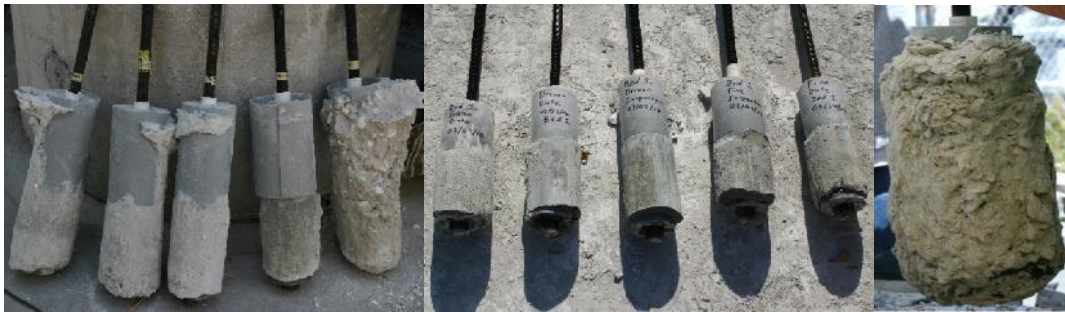
Figure 4.19. Extracted sockets from bed 5 (left), bed 1 (center) and bed 4 (right).
