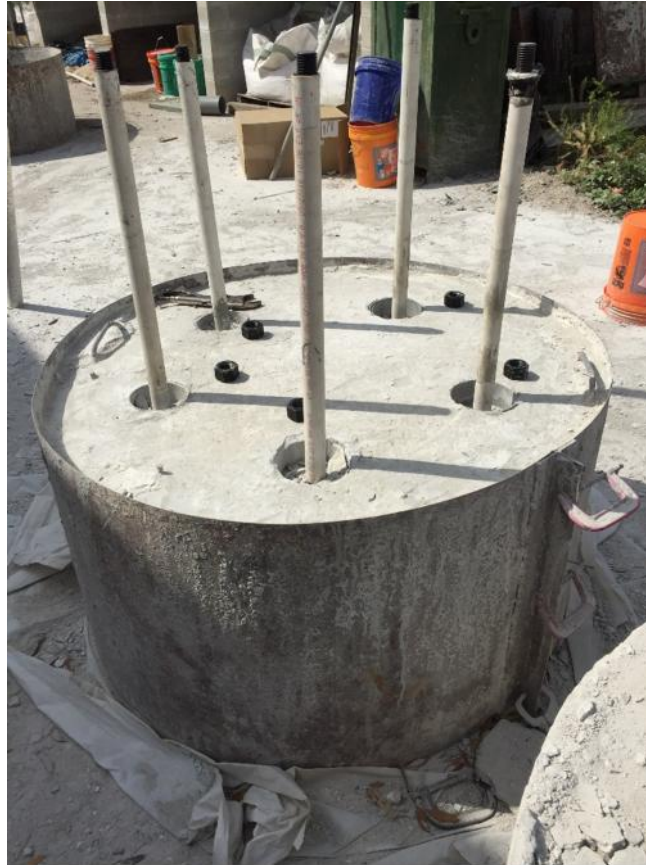
Figure 5.6. Rock socketed specimens being prepared for pull-out tests.
