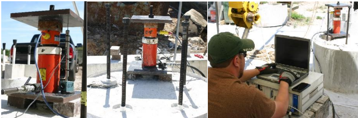
Figure 4.18. Pull-out load test in progress.
