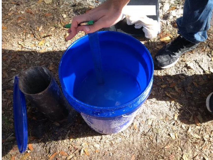
Figure 3.24. Volumetric measurement of the slurry being introduced in the shafts (phase 2).
