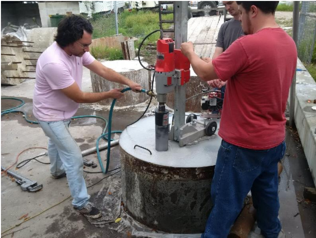
Figure 4.8. Top of simulated limestone beds flooded with water and being pre-cored.
