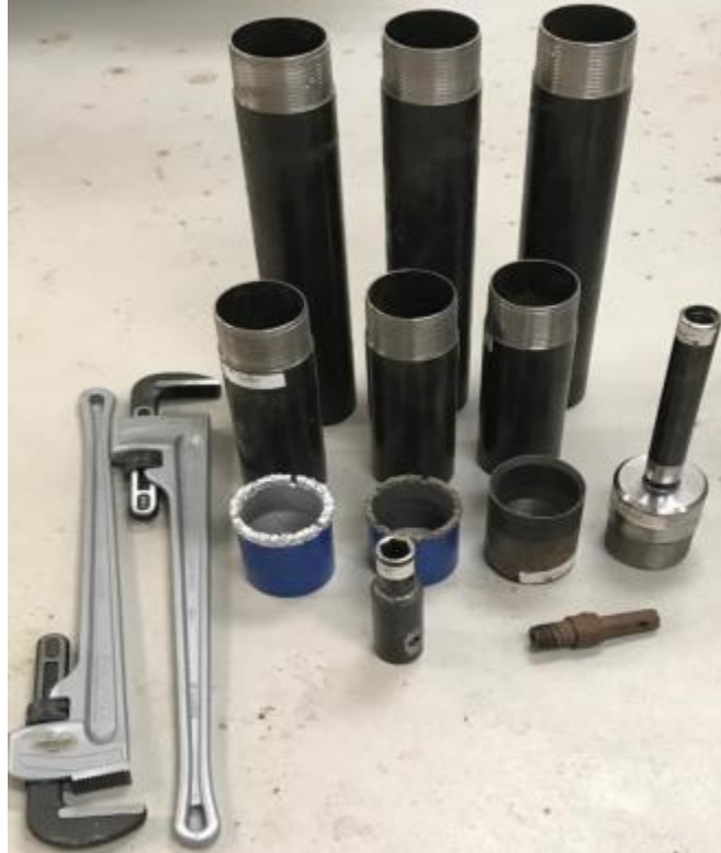
Figure 4.6. Casing cutting tips, drive shoe, casing extensions and drill rod couplers.
