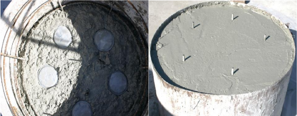
Figure 4.3. Debonding plastic disks (left) and centering rods (right).
