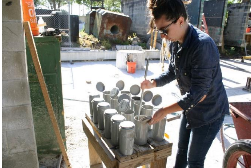
Figure 4.4. Preparation of cylinders from limestone bed material.
