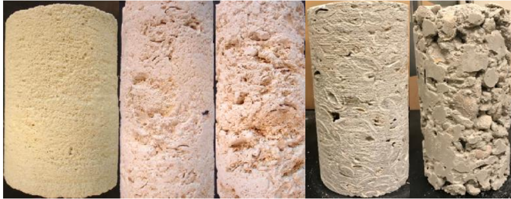
Figure 4.1. Field retrieved limestone cores (left); core from simulated limestone bed and simulated limestone cylinder specimen (right).
