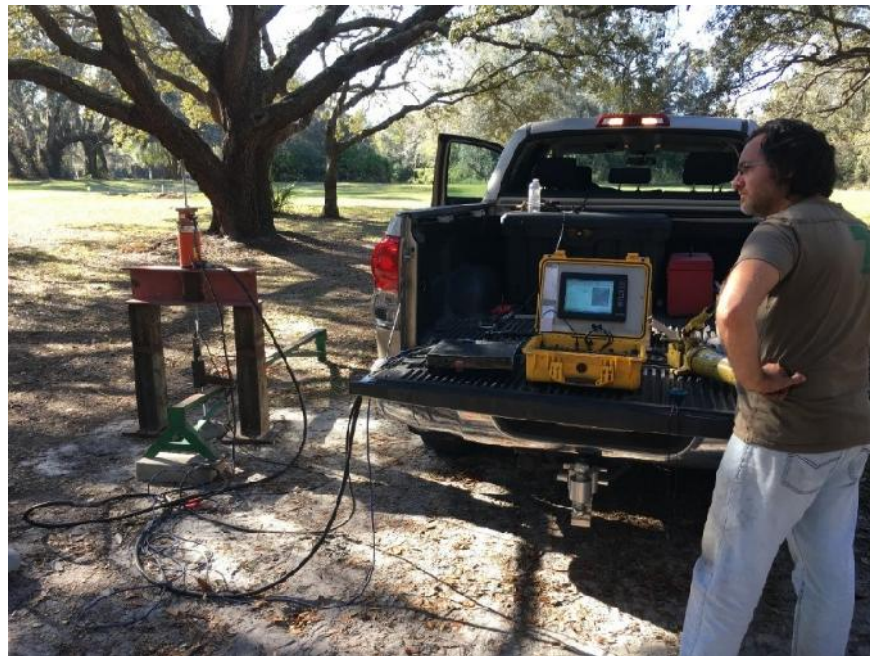
Figure 3.15. Small-scale pull-out load tests setup.
