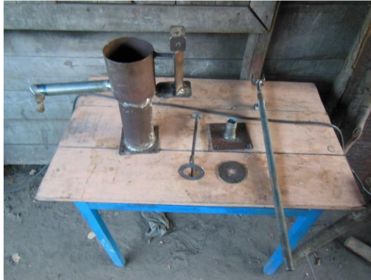
Figure 1.3 Pitcher Pump assembly from a Morondava workshop (excluding both check valves). (Photo from the author.)
