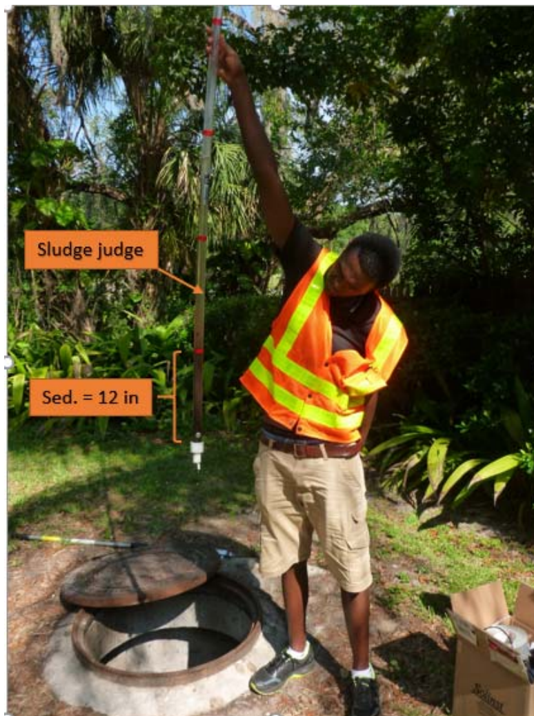
Figure 3-2: Sludge-judge in operation
