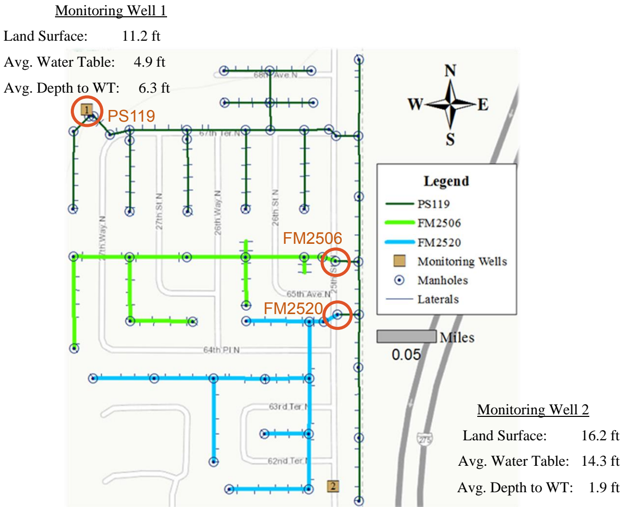
Figure 12: Layout of flowmeters, corresponding sewersheds, and monitoring wells. (Land surface elevations in ft. NAVD)
