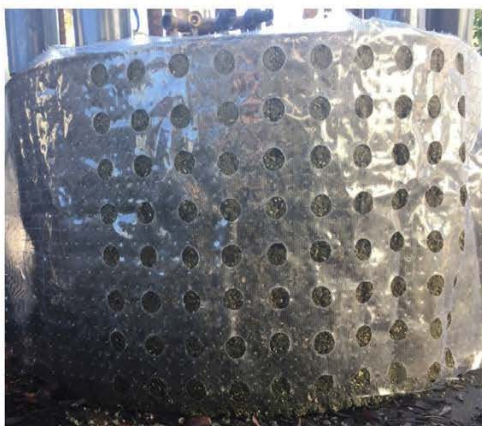
Figure 4.25 Shaft 24 testing template and corrosion potential map
