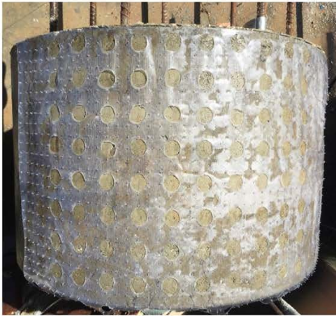
Figure 4.21 Shaft 20 testing template and corrosion potential map
