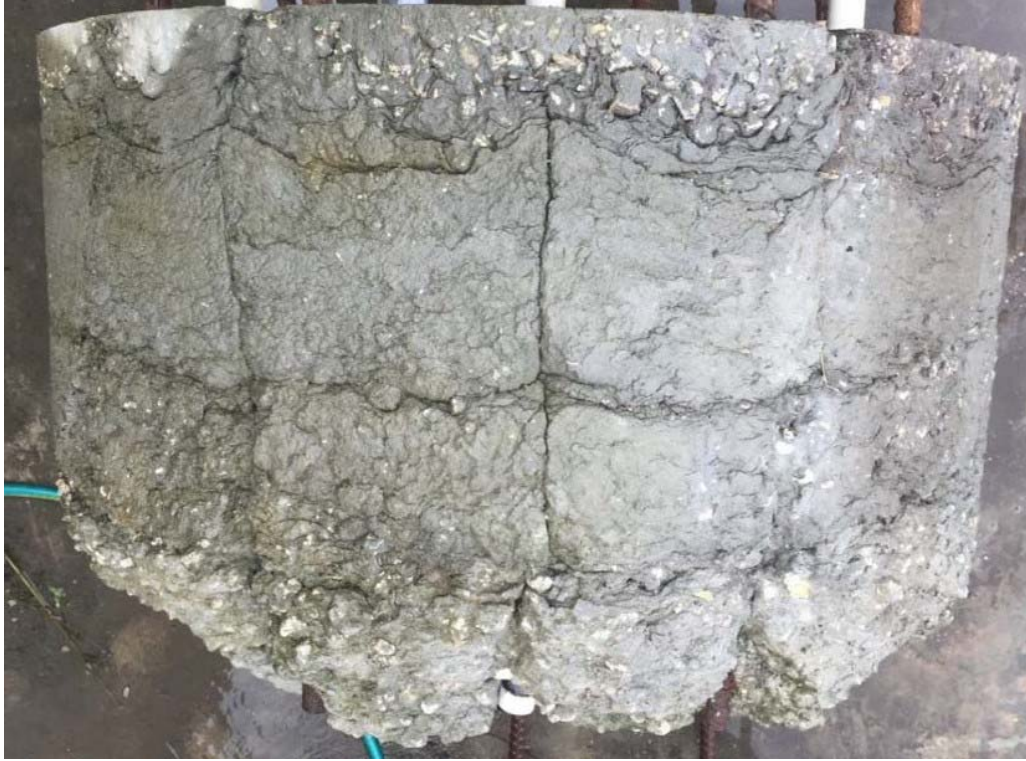
Figure 1.3 Quilting in a drilled shaft experimental specimen
