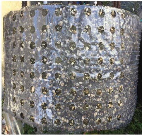
Figure 4.9 Shaft 7 testing template and corrosion potential map
