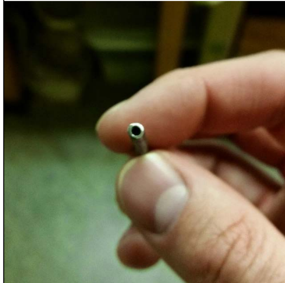
Figure 3.14 Drilled out titanium rod
