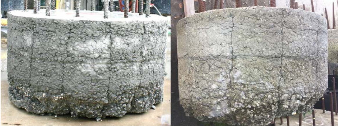
Figure 2.16 Shaft 10: f'c 4530 psi; drilled shaft mix, 50 sec/qt bentonite; rough with defined creases
