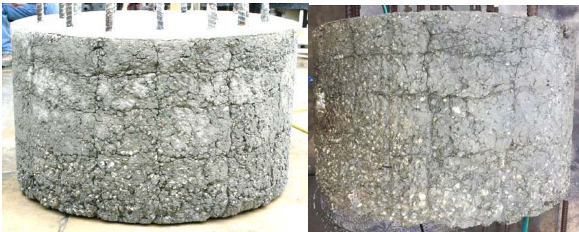
Figure 2.15 Shaft 9: f'c 4530 psi; drilled shaft mix, 50 sec/qt bentonite; rough with defined creases
