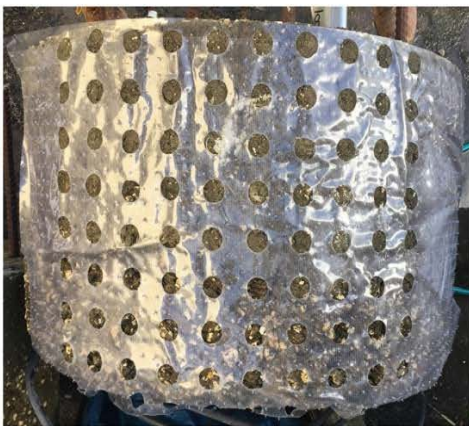
Figure 4.10 Shaft 8 testing template and corrosion potential map
