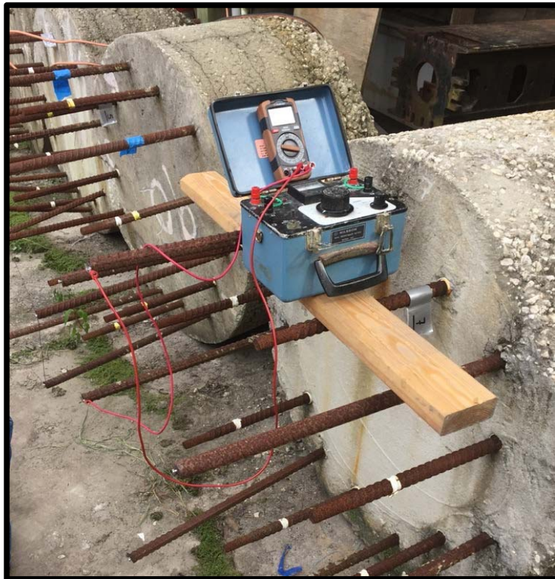
Figure 3.4 Mutual potential / mutual resistance testing setup
