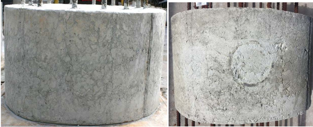
Figure 2.22 Shaft 16: f'c 4753 psi; drilled shaft mix, 85 sec/qt polymer, smooth light creases
