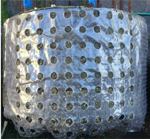
Figure 4.5 Shaft 3 testing template and corrosion potential map
