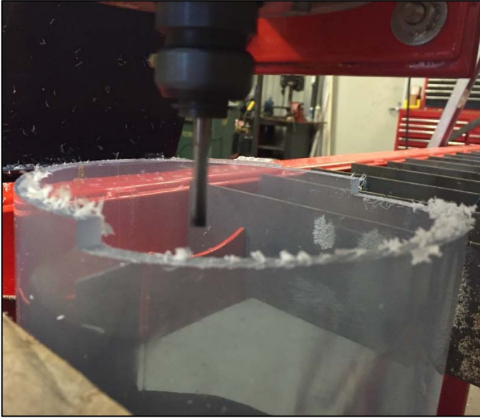
Figure 3.10 Rounding end of tank
