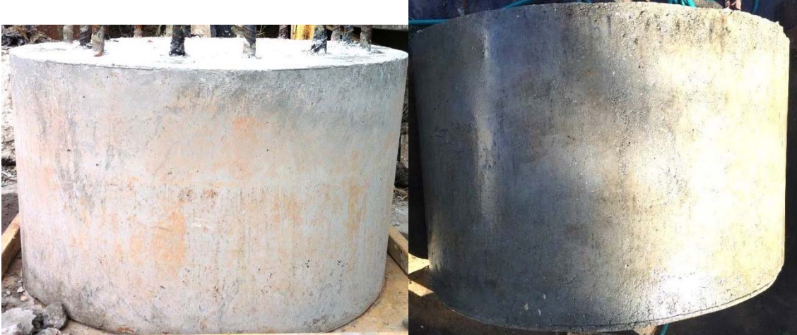
Figure 2.25 Shaft 19: f'c 4100 psi; drilled shaft mix, 63 sec/qt polymer, smooth
