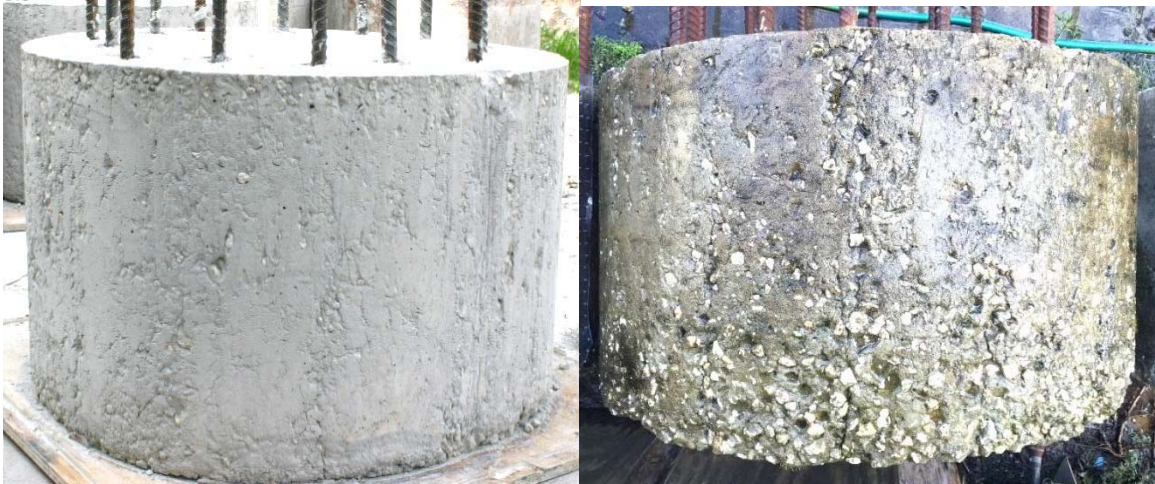
Figure 2.19 Shaft 13: f'c 4753 psi; drilled shaft mix, 30 sec/qt bentonite, rough
