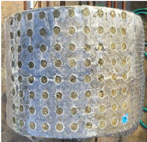
Figure 4.17 Shaft 16 testing template and corrosion potential map
