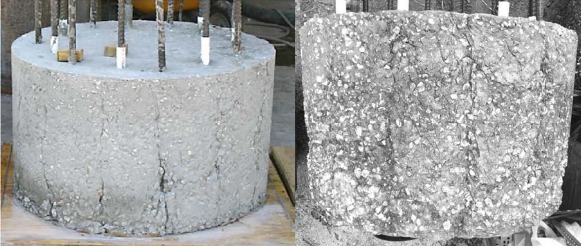
Figure 2.7 Shaft 1: f'c 6150psi; drilled shaft mix; 44 sec/qt bentonite; rough with creases
