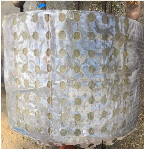
Figure 4.23 Shaft 22 testing template and corrosion potential map
