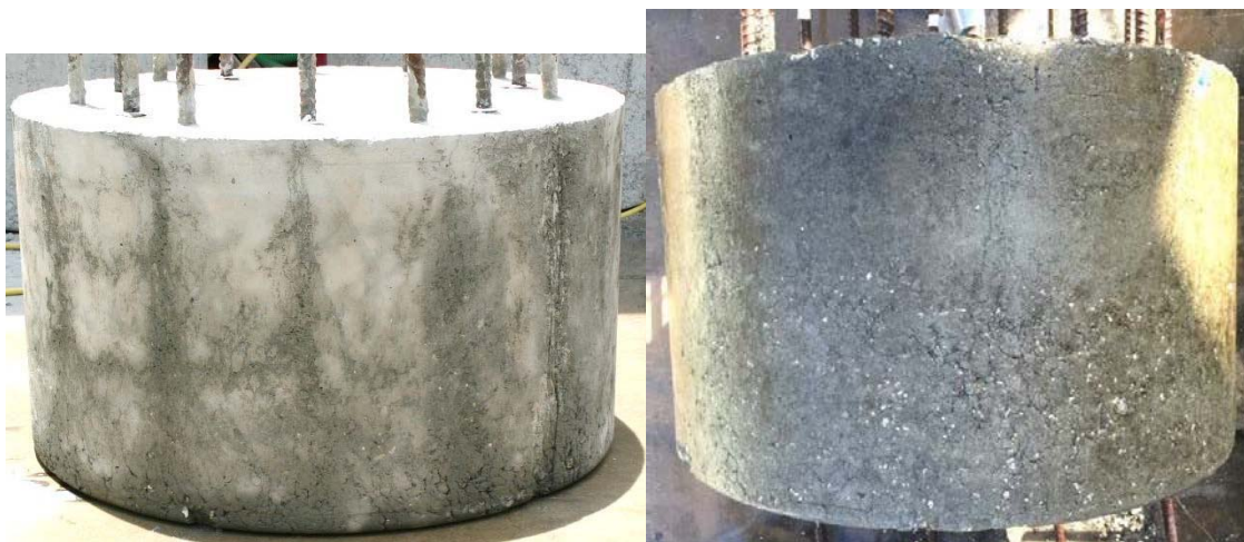
Figure 2.18 Shaft 12: f'c 4530 psi; drilled shaft mix, drilled shaft mix, 66 sec/qt polymer, rough
