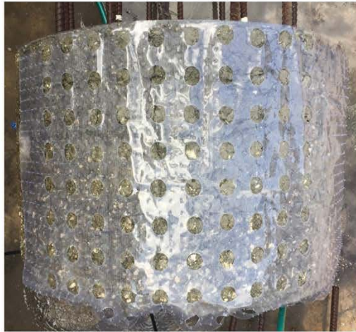
Figure 4.11 Shaft 9 testing template and corrosion potential map
