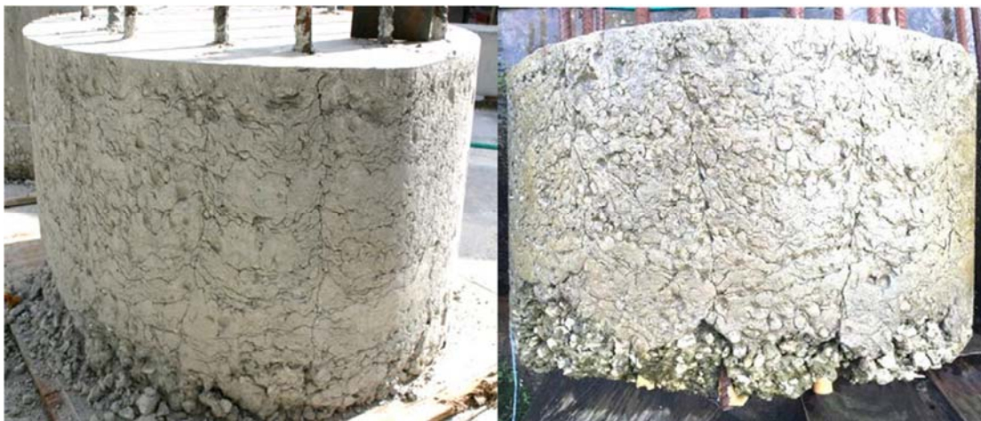
Figure 2.21 Shaft 15: f'c 4753 psi; drilled shaft mix, 56 sec/qt bentonite, rough with defined creases
