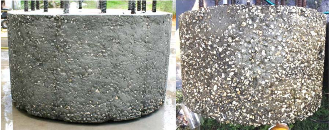
Figure 2.13 Shaft 7: f'c 4530 psi; drilled shaft mix, 30 sec/qt bentonite; coarse.
