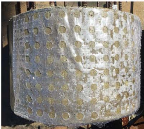
Figure 4.19 Shaft 18 testing template and corrosion potential map
