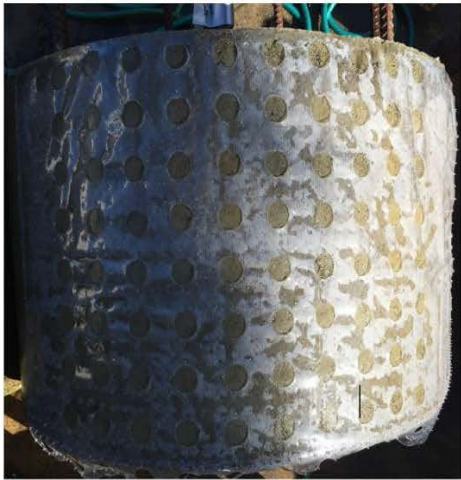
Figure 4.20 Shaft 19 testing template and corrosion potential map
