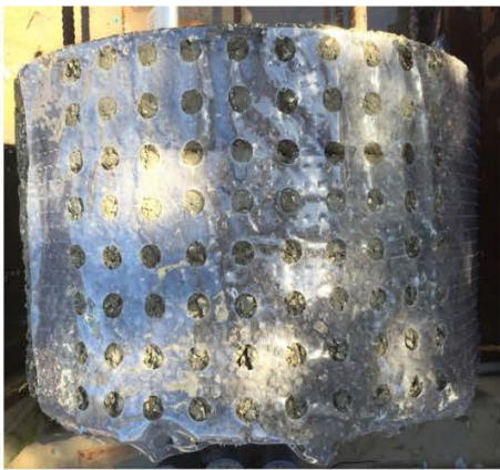
Figure 4.22 Shaft 21 testing template and corrosion potential map
