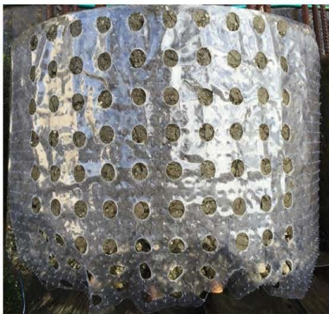
Figure 4.16 Shaft 15 testing template and corrosion potential map
