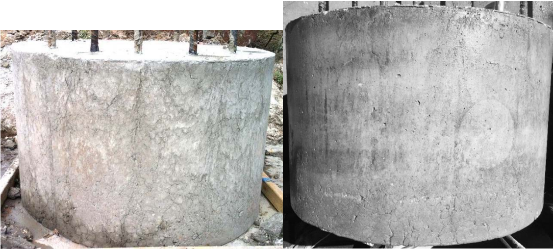
Figure 2.26 Shaft 20: f'c 4100 psi; drilled shaft mix, 121 sec/qt polymer, smooth
