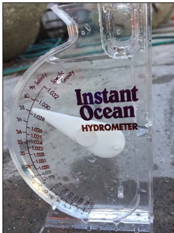
Figure 3.20 Hydrometer used to test specific gravity
