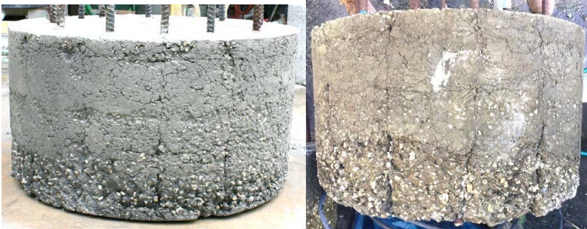
Figure 2.14 Shaft 8: f'c 4530 psi; drilled shaft mix, 40 sec/qt bentonite; rough with defined creases
