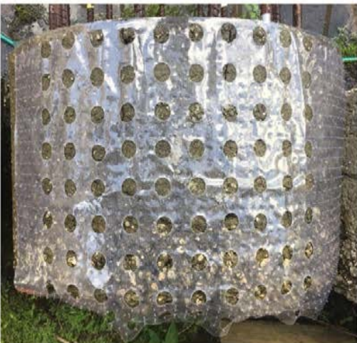
Figure 4.7 Shaft 5 testing template and corrosion potential map
