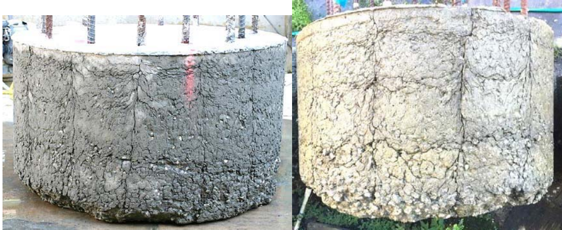
Figure 2.9 Shaft 3: f'c 4358 psi; drilled shaft mix; 40 sec/qt bentonite; coarse with well-defined creases.
