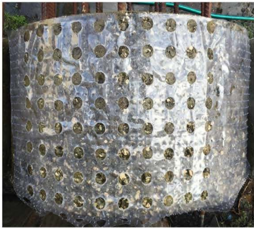
Figure 4.14 Shaft 13 testing template and corrosion potential map
