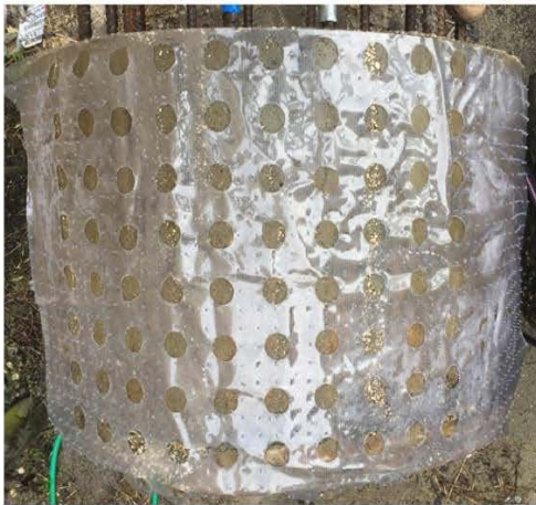
Figure 4.24 Shaft 23 testing template and corrosion potential map
