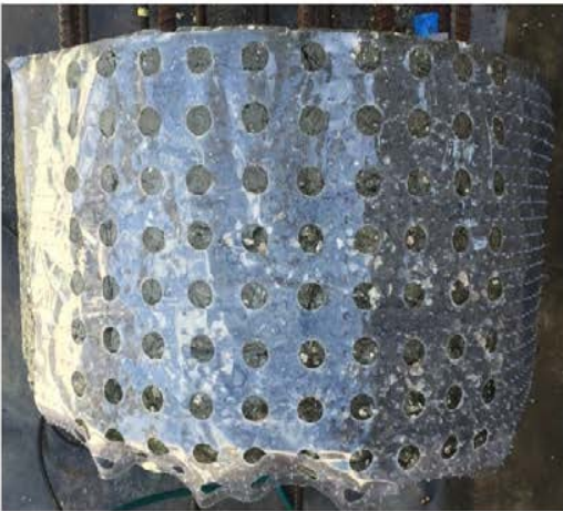
Figure 4.6 Shaft 4 testing template and corrosion potential map
