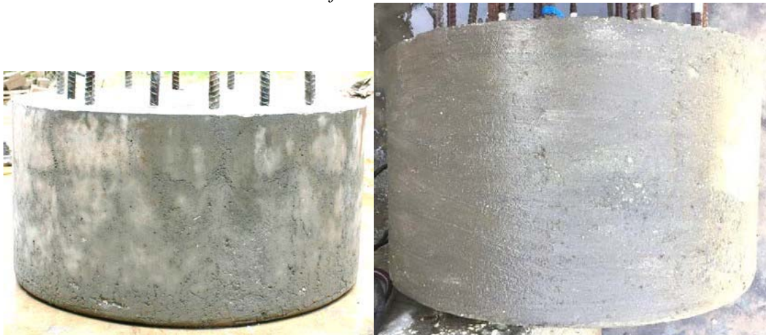
Figure 2.16 Shaft 10: f'c 4530 psi; drilled shaft mix, 50 sec/qt bentonite; rough with defined creases
