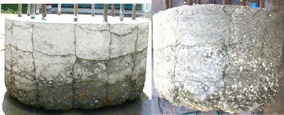
Figure 2.10 Shaft 4: f'c 4358 psi; drilled shaft mix; 55 sec/qt bentonite; coarse with well-defined creases.
