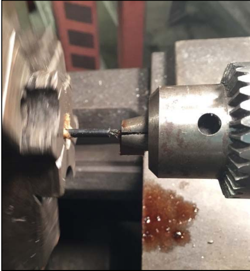
Figure 3.13 Drilled titanium rod
