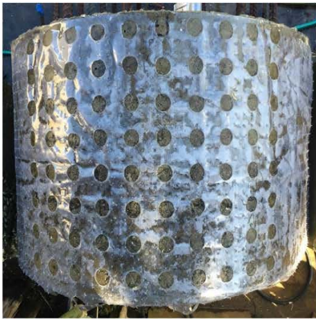
Figure 4.18 Shaft 17 testing template and corrosion potential map
