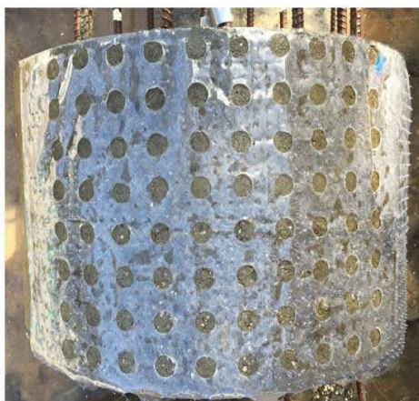
Figure 4.13 Shaft 12 testing template and corrosion potential map
