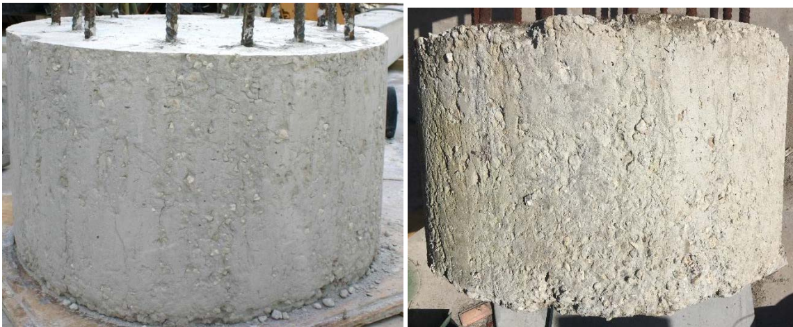
Figure 2.20 Shaft 14: f'c 4753 psi; drilled shaft mix, 30 sec/qt bentonite, rough
