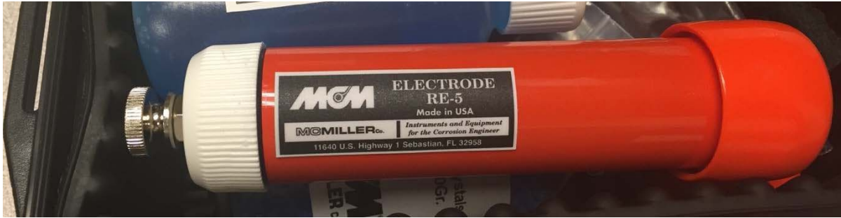
Figure 3.8 Copper- copper sulfate reference electrode
