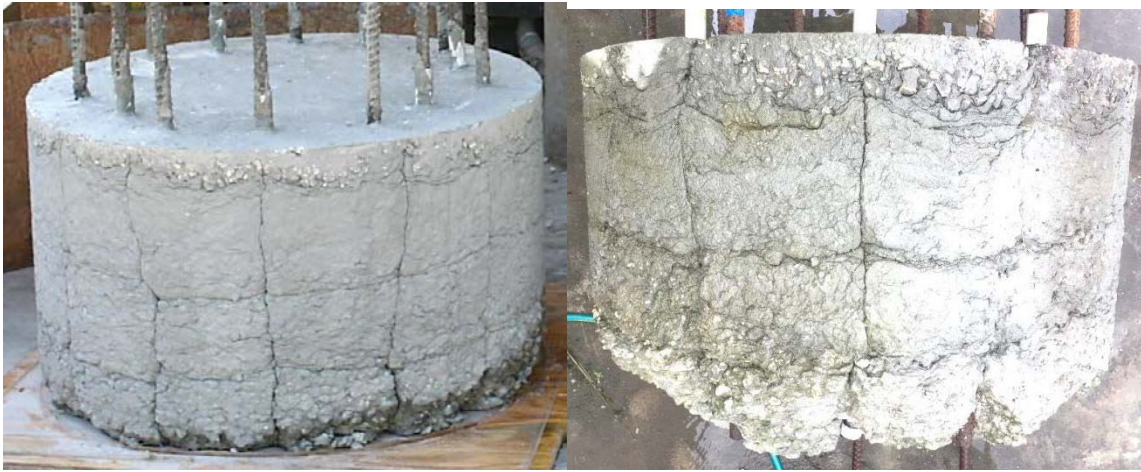
Figure 2.8 Shaft 2: f'c 6150psi; drilled shaft mix; 105sec/qt bentonite; coarse with well-defined creases
