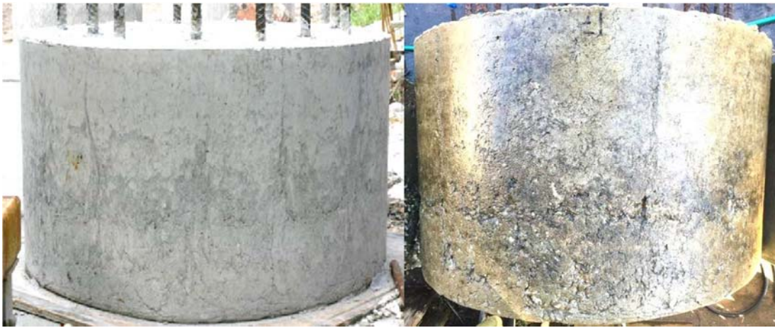
Figure 2.23 Shaft 17: f'c 4753 psi; drilled shaft mix, 85 sec/qt polymer, smooth light creases
