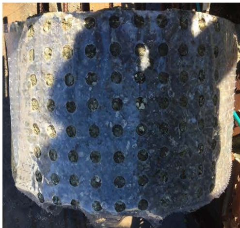
Figure 4.15 Shaft 14 testing template and corrosion potential map
