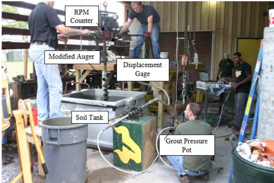
Figure 3.9. Wet mixing machine design (Baker, 2015).
