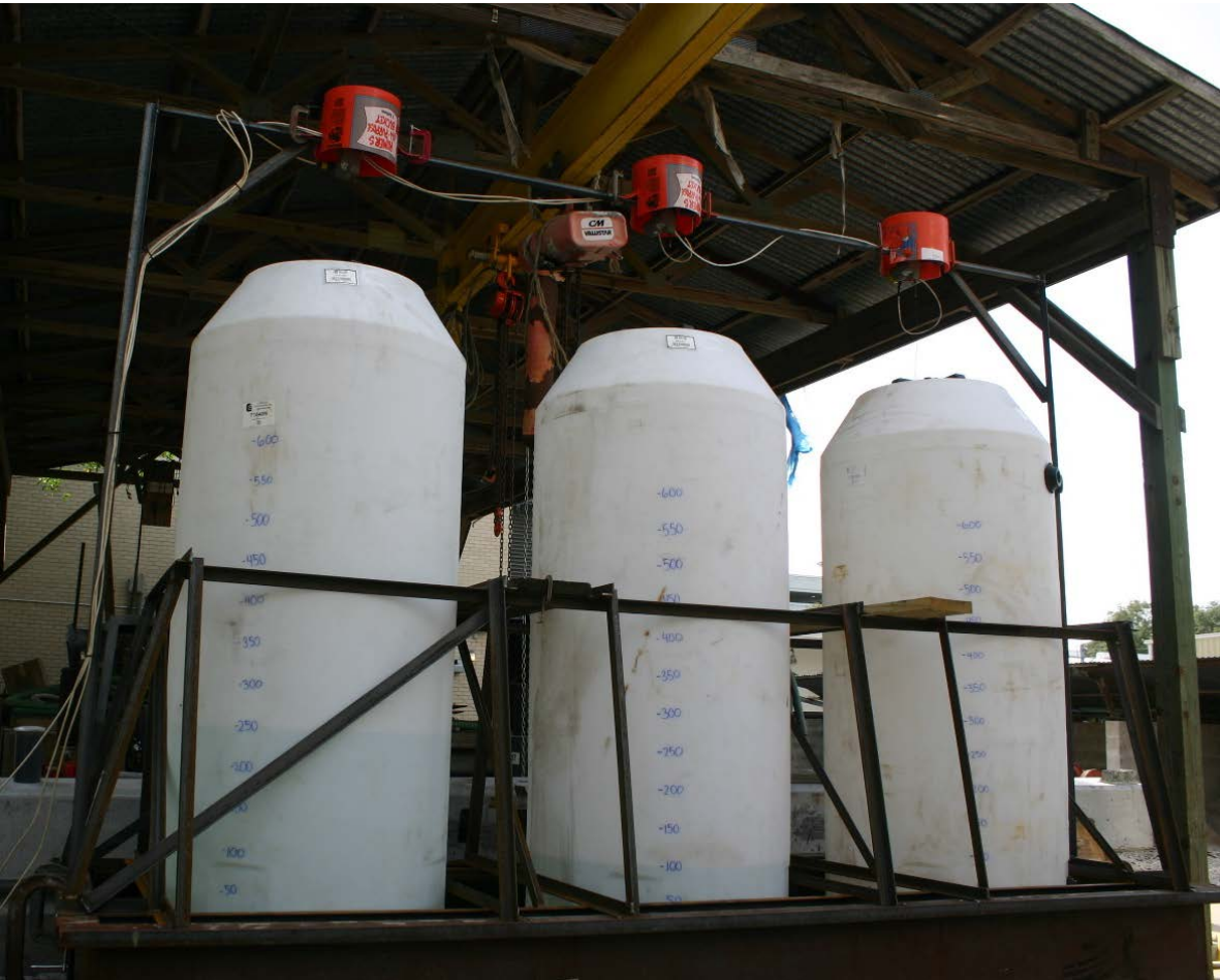
Figure 3.24. Loading system on the test bed.
