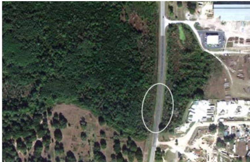
Figure 4.1 Aerial view of a 1000ft section of SR 33 north of Polk City, FL that has been continuously repaired to combat subsidence. Denoted region represents worst area.
