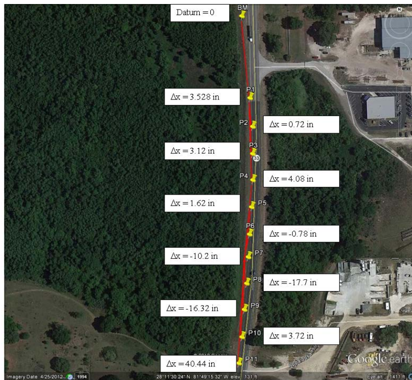
Figure 4.5. Initial survey measurements along SR 33 just north of Polk City.
