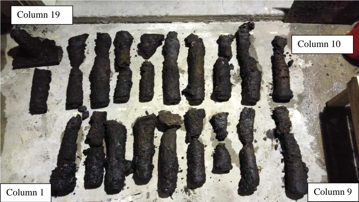
Figure 3.32. The 19 wet-mixed columns after excavation.
