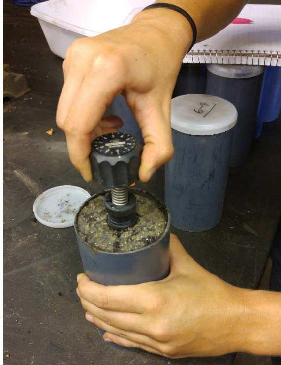
Figure 3.6. Vane shear test performed on the slag-cement cylinders.
