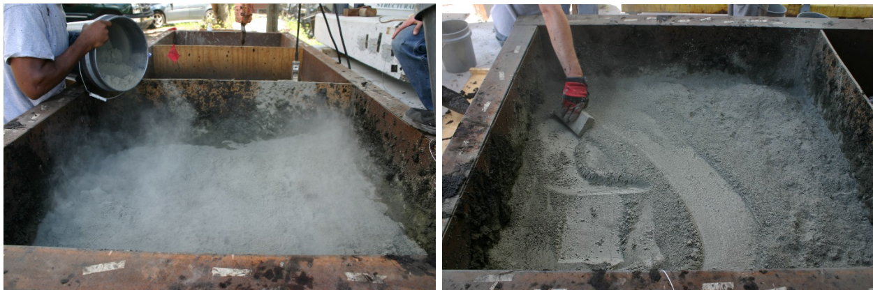
Figure 3.18. Adding of cement (left), and making sure it was equally distributed (right).
