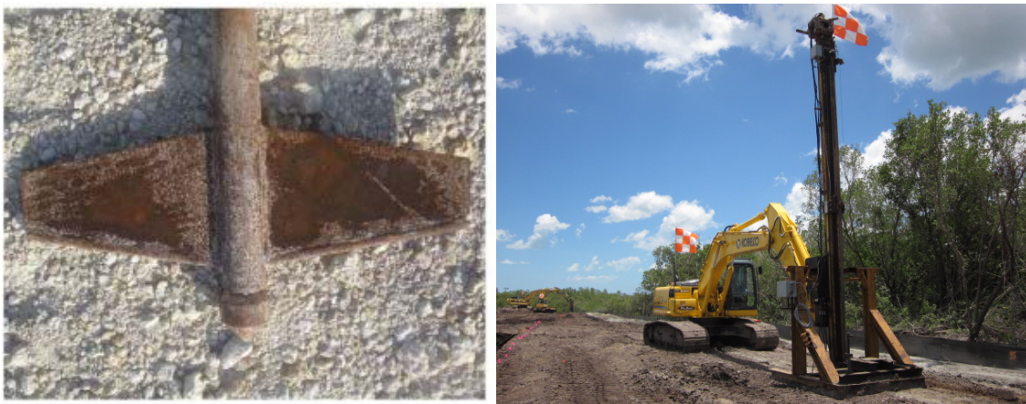
Figure 4.9. KPS penetrometer with load distribution wings (left); and KPS thrusting unit (right).
