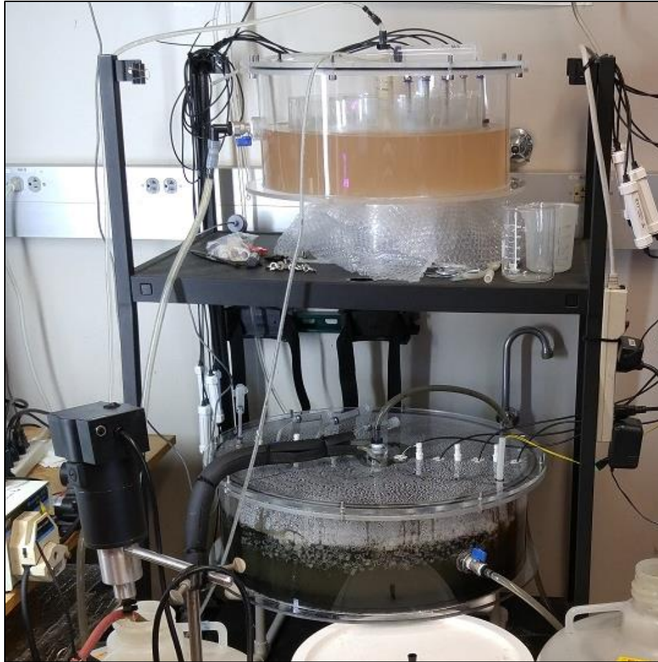
Figure 3.11. The large (bottom) and small (top) CBR prototypes
