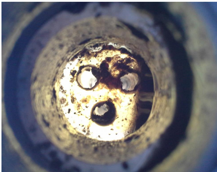
Figure 4.11: Feed side view of M2 after it was removed from the testing system. The foulant layer, visible as a brown stain can be seen running the length of the membrane module.
