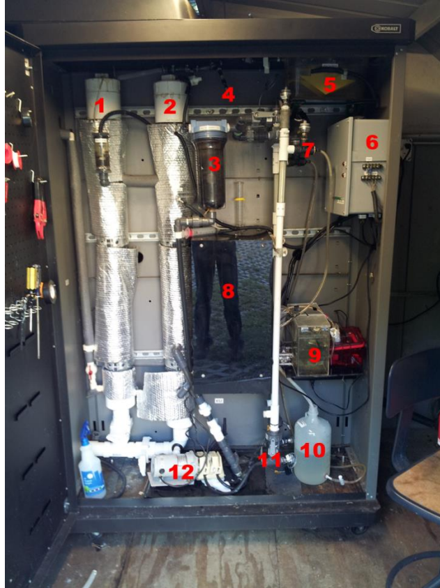
Figure A2: Front view of AnMBR system as built and tested in chapters 3 and 4.
