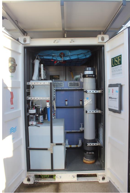
Figure C2: Doors open on the TRL 7 system. In the background the ABR can be seen, while in the foreground on the left the chlorination tank and system
