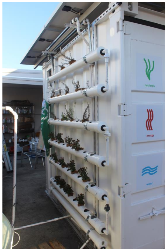
Figure C1: TRL 7 unit with incorporated hydroponics being hydraulically tested at the USF's Tampa Campus.
