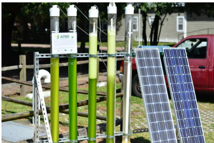
Figure A5: Algal photobioreactors located at the entrance of the shed containing the TRL 6 AnMBR. Permeate from the system was used for this demonstration unit for algal growth.
