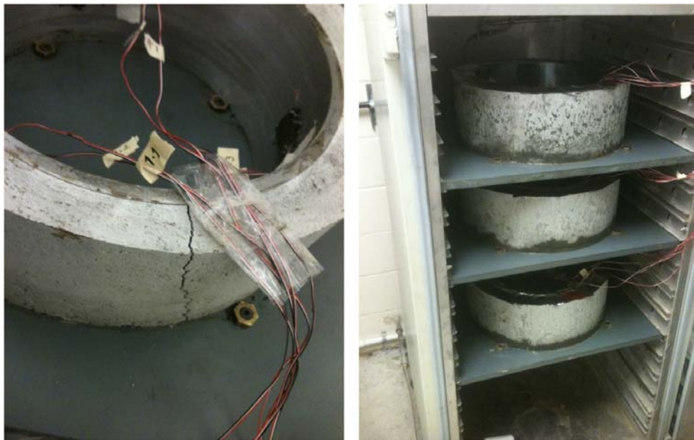
Figure 5.3 Restrained shrinkage ring specimens
