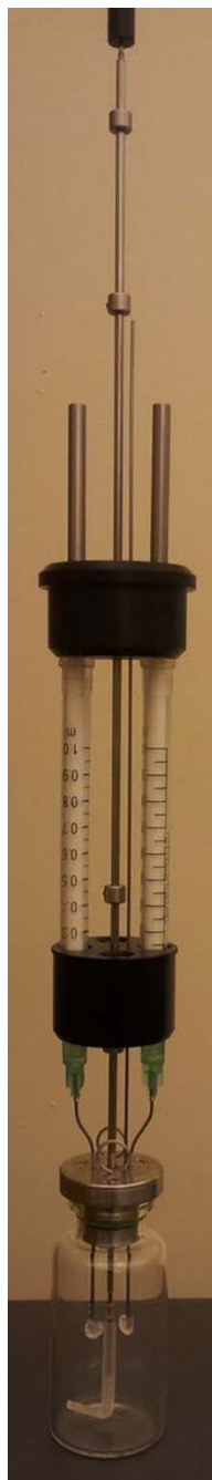
Figure 2.1 Admixer and vial for internal mixing (isothermal conduction calorimetry)
