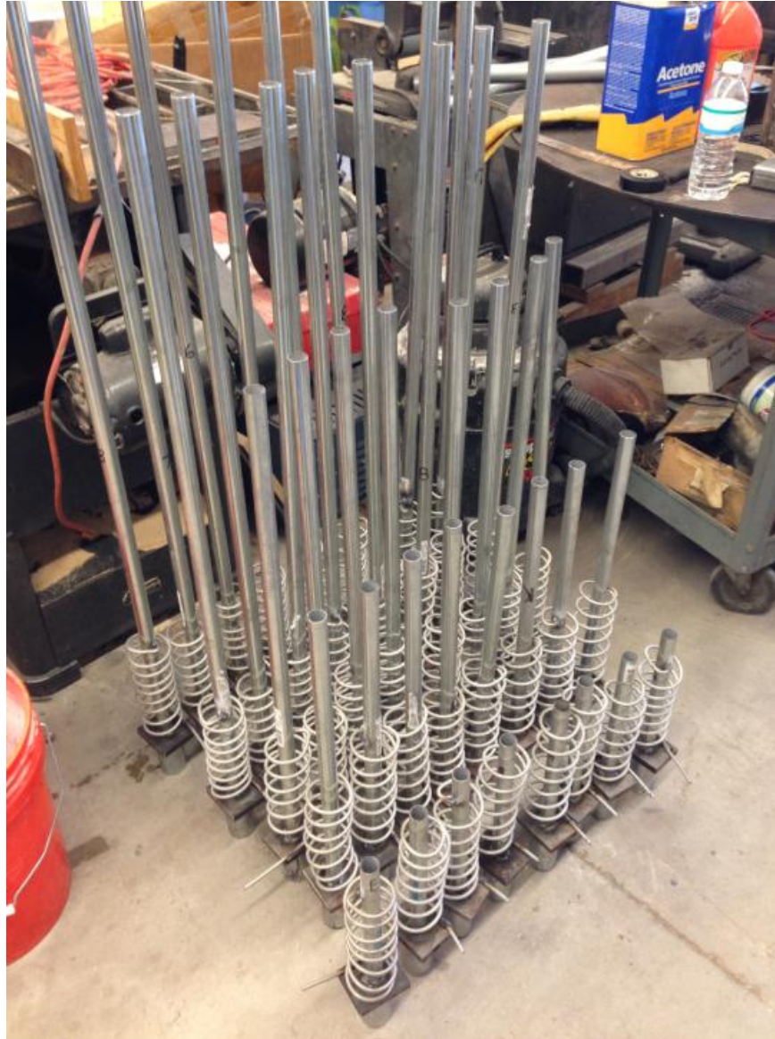
Figure 4.3 Finished internal splicing components.
