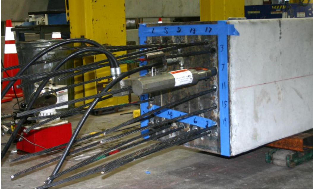
Figure 4.8 Jacking orders of strands
