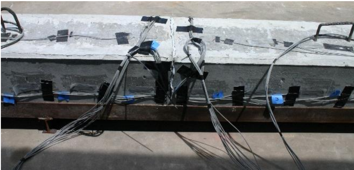
Figure 2.4 Photo of finished strain gage layout.
