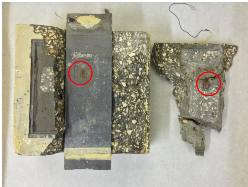
Figure E.10 Corrosion spots on the steel-concrete interface of specimen S4
