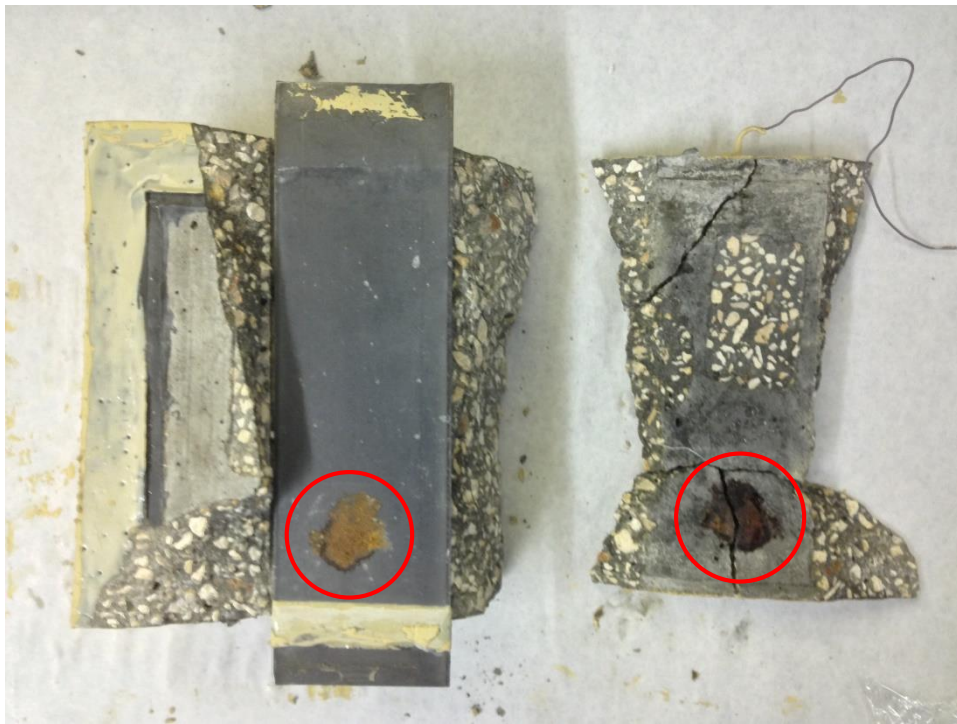
Figure E.8 Corrosion spots on the steel-concrete interface of specimen M7
