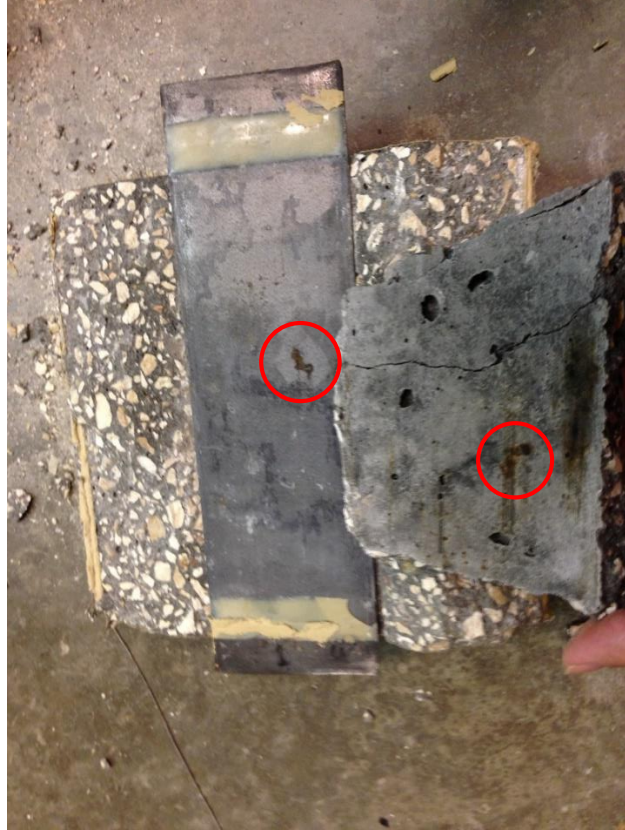
Figure E.1 Corrosion spots on the steel-concrete interface of specimen C1.
