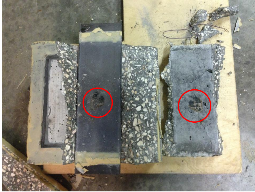
Figure E.9 Corrosion spots on the steel-concrete interface of specimen M11
