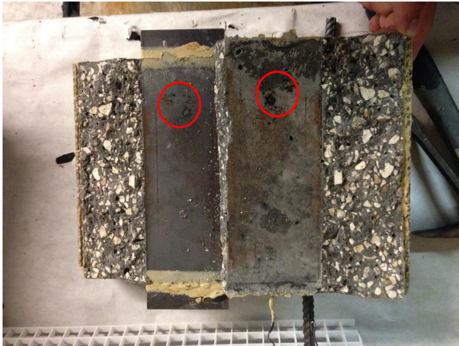
Figure E.3 Corrosion spots on the steel-concrete interface of specimen C9
