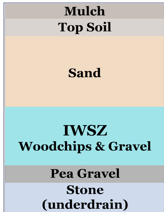
Figure 1.1b. Diagram of a Modified Bioretention Cell
