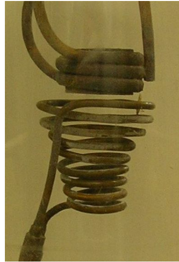
(b) Detail of levitation cell coil.
