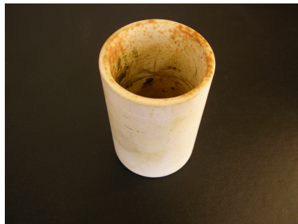
(c) Crucible after use in experiments with vanadium at 600°C.
