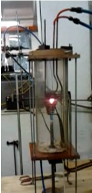
(a) Levitation cell in operation.
