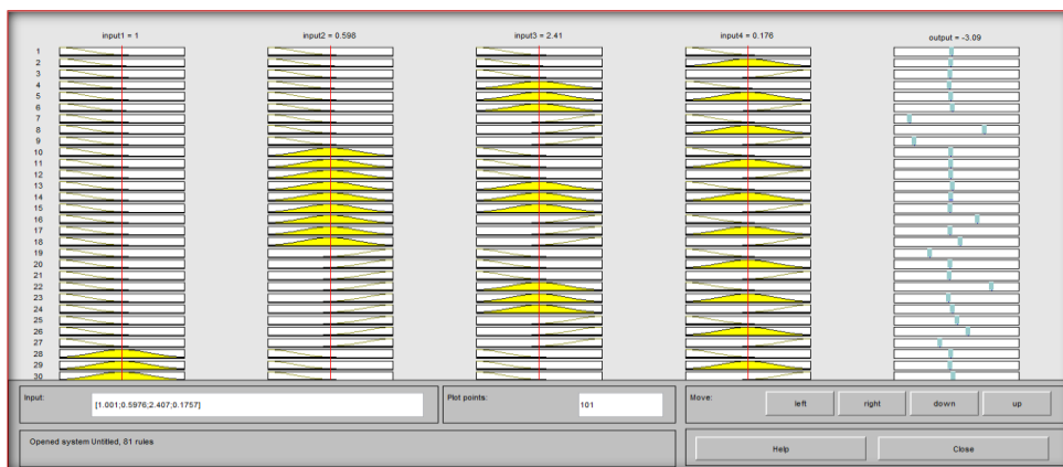
Figure 5.61 A sample set of rules by rule viewer for prediction of WQI entrance length for winter
