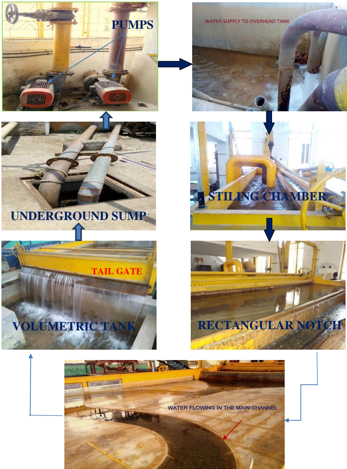
Figure 7 Flow Chart of the Water Supply System
