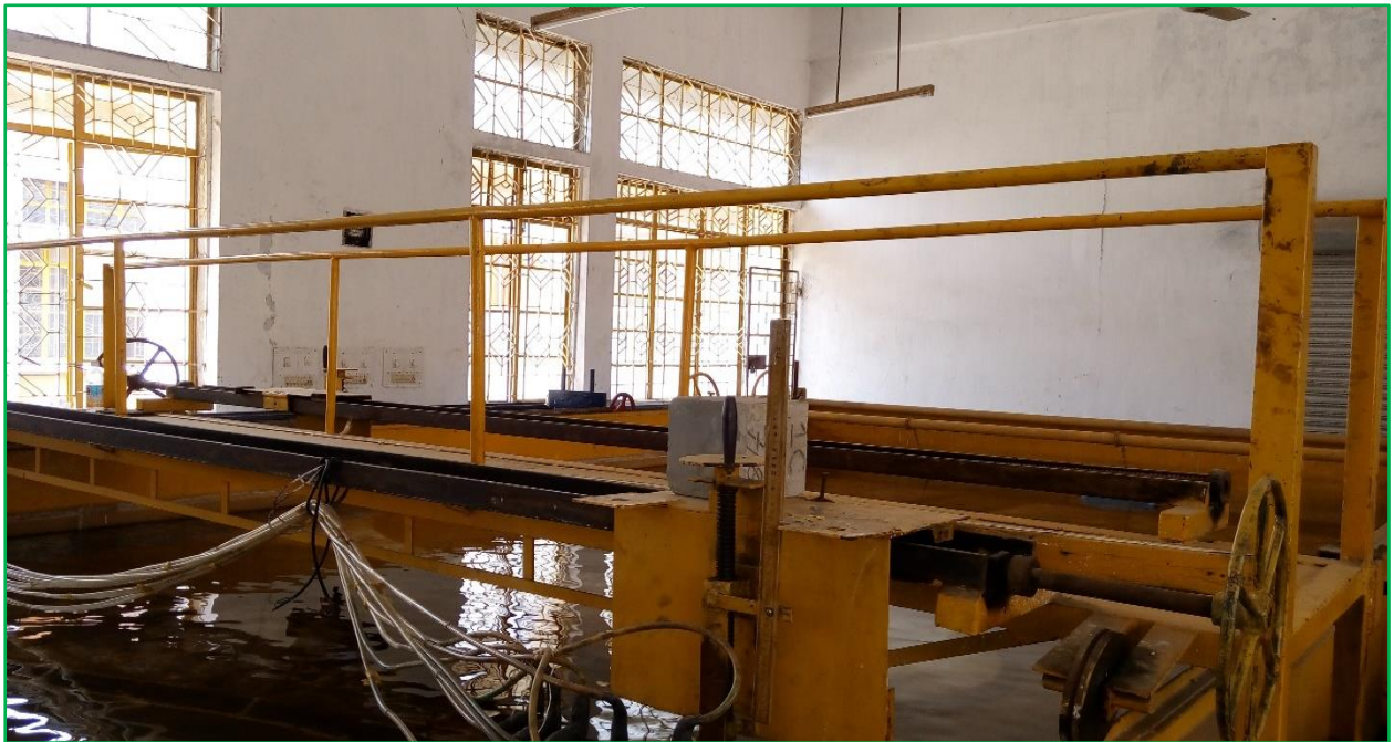
Figure 8.5 Moving Bridge Arrangement
