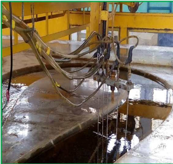
Figure 17 Photograph during Velocity Measurement
