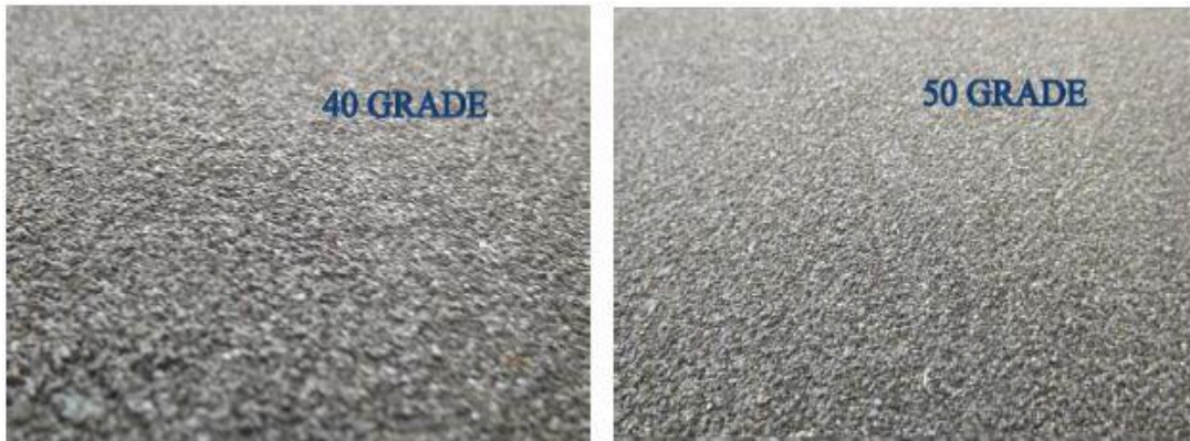
Fig. No. 4.3.3(a) Rough surfaces of grade 40(375 \mu m) and 50(345 \mu m)
