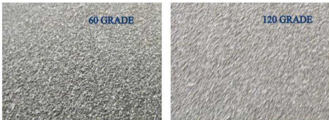
Fig. No. 4.3.3(b) Rough surfaces of grade 60(290 \mu m) and 120(125 \mu m)
