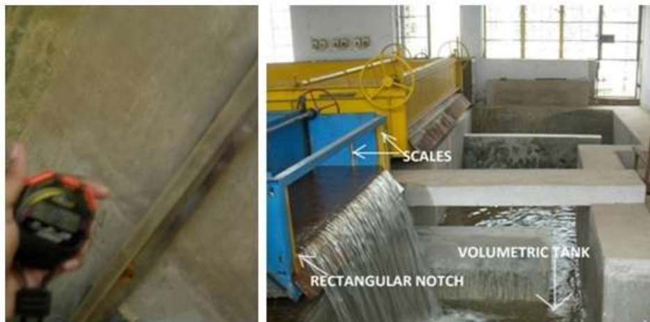
Fig. 3.5 Rectangular-Notch calibration experiment
