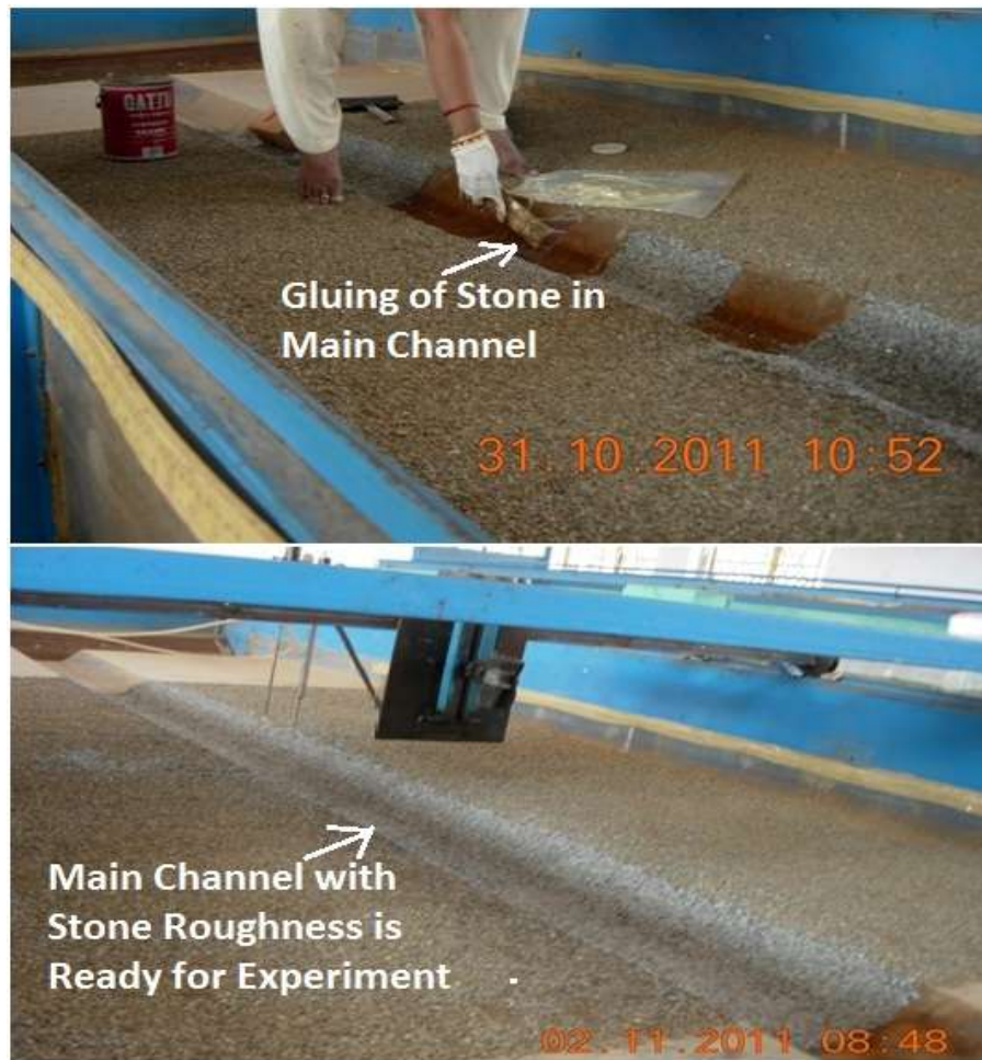
Fig. 3.12 Constriction of stone roughened main channel
