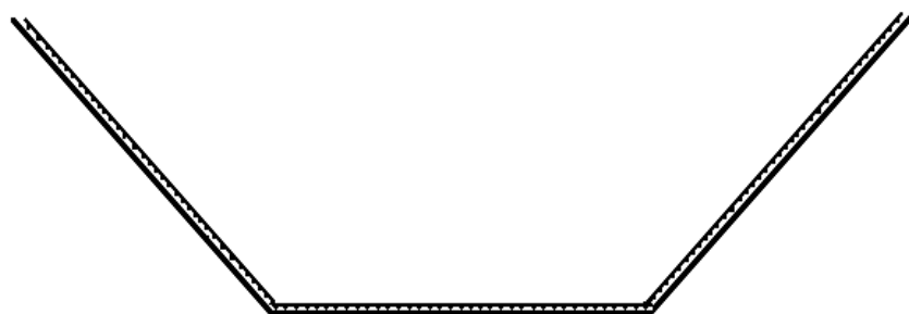
Fig. 3.9 Schematic drawing of the mesh roughened main channel cross-section
