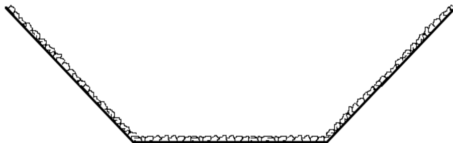
Fig. 3.11 Schematic drawing of the stone roughened main channel cross-section
