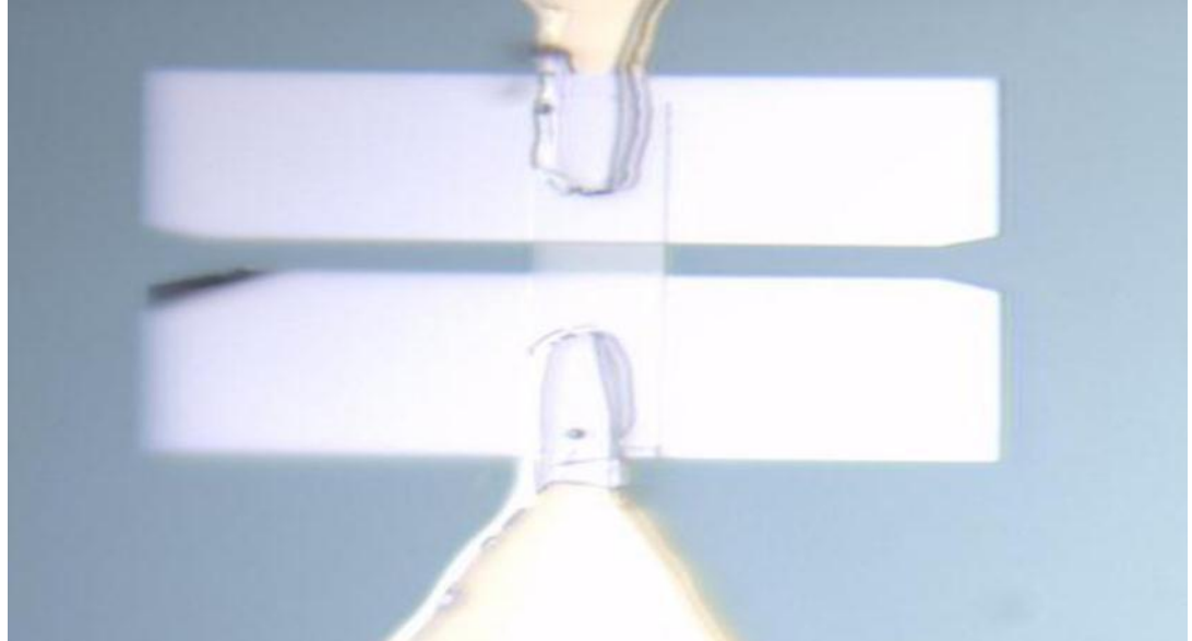
Figure 2.11: Nb bolometer of 1.5\mu\text{m} \times 5\mu\text{m} dimensions
