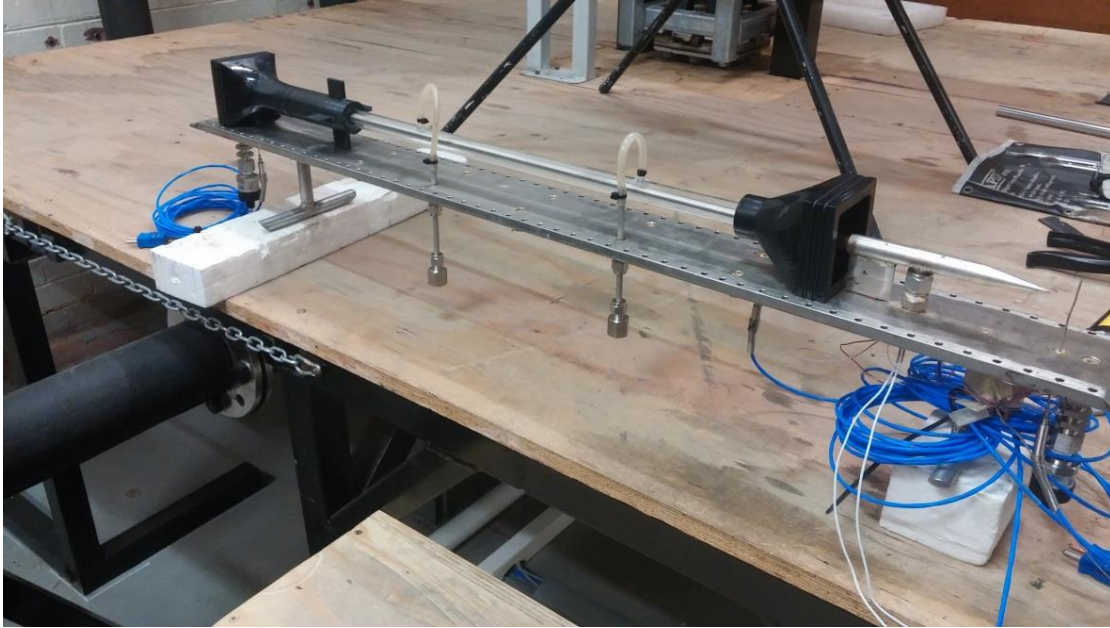
Figure 23 Inlet and outlet flow concentrators
