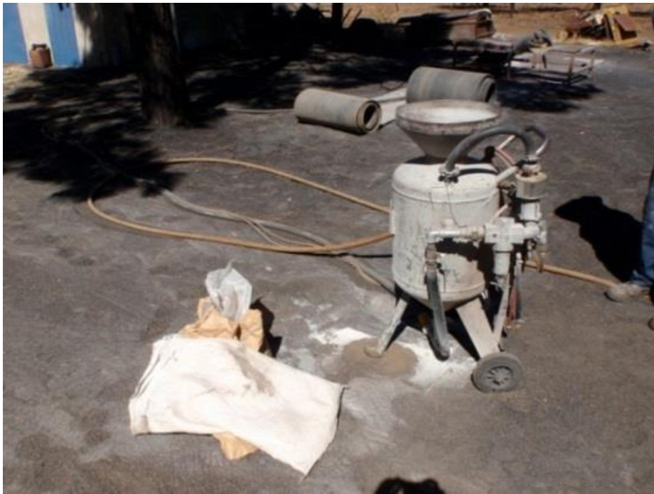
Figure 17 Sandblasting equipment used
