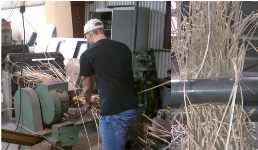
Figure 3-1: Switchgrass nodes being crushed using sheet metal rollers
