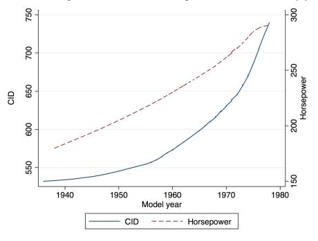
Figure B.1: Relationship between CID and horsepower - data from survey year 1977
