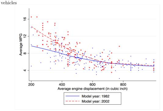
Figure 2.5: Trade-off between MPG and engine displacement for class 3-8 vocational
