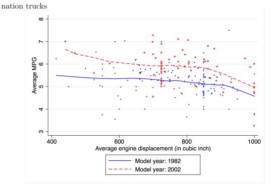
Figure 2.3: Trade-off between MPG and engine displacement for class 7, 8 combi-
