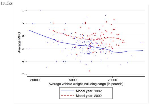
Figure 2.2: Trade-off between MPG and vehicle weight for class 7, 8 combination
