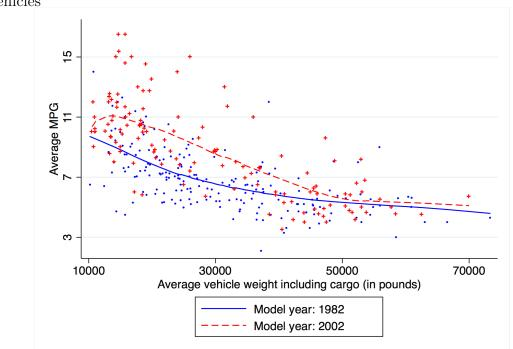
Figure 2.4: Trade-off between MPG and vehicle weight for class 3-8 vocational vehicles
