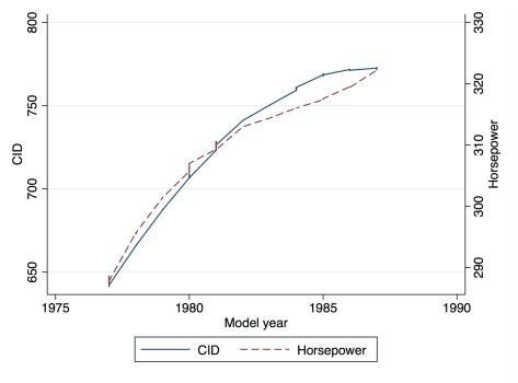
Figure B.3: Relationship between CID and horsepower - data from survey year 1987
