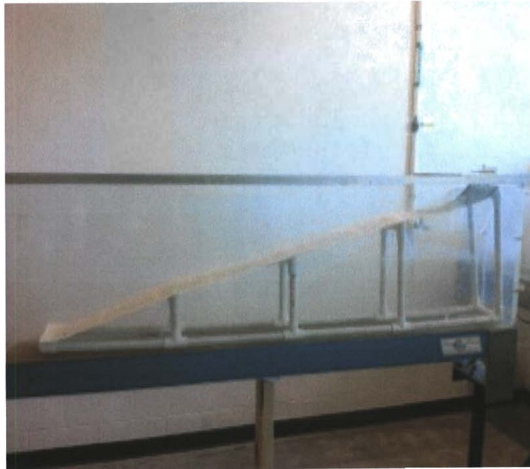
Figure 3.7 Ramp at end of the tank used to eliminate reflection off end wall
