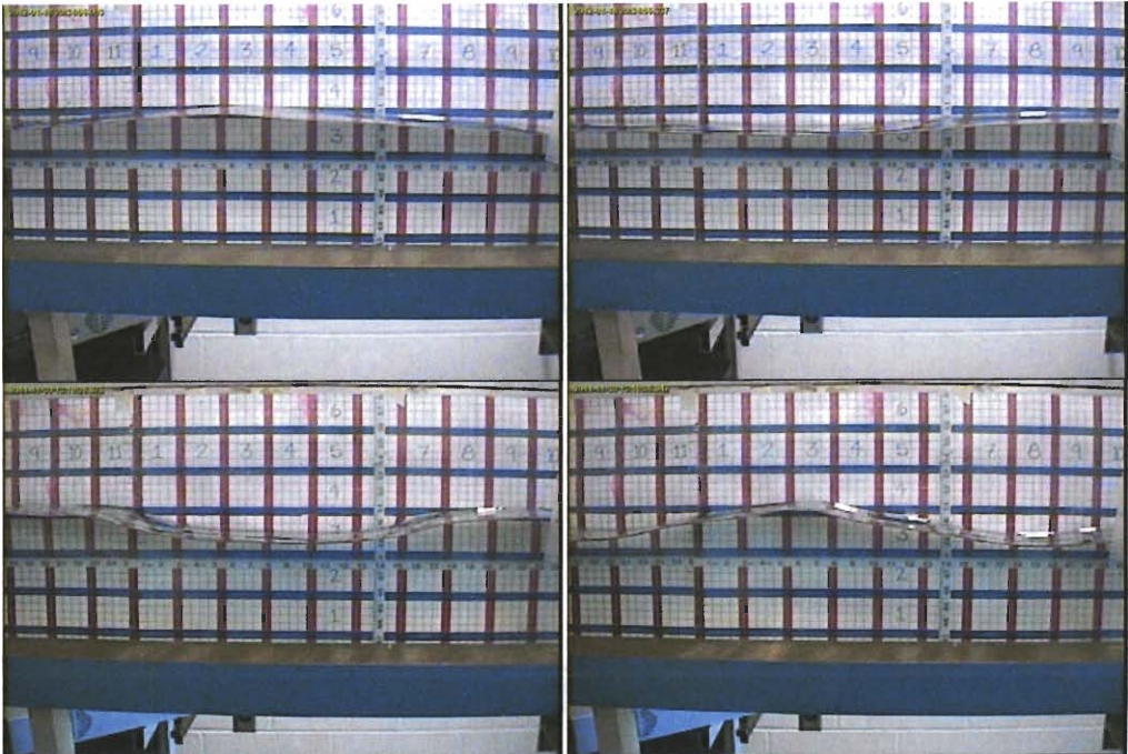
Figure A.5 Wave without 3-D effect in WMU wave tank
