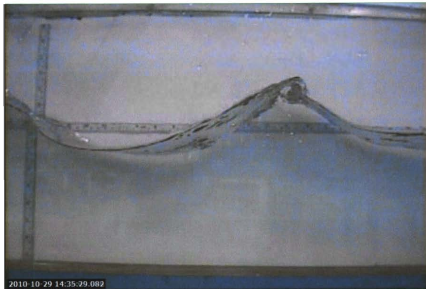
Figure A.3 3-D effect of the higher frequency waves of waves in WMU wave tank
