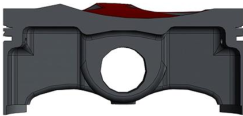
High Compression Shallow Bowl Piston Design (Modified pentroof surface with 3mm deep bowl)
