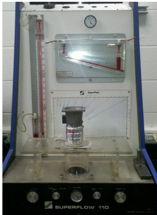
Figure 27. Flow sensor calibration setup using a flow bench
