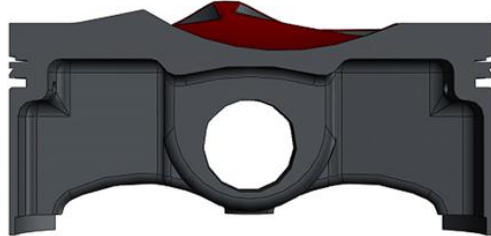
High Compression Deep Bowl Piston Design (Modified pentroof surface with 6mm deep bowl)
