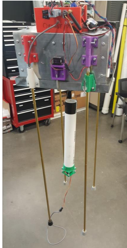
Figure 25: Ballast Connected to Sampler
