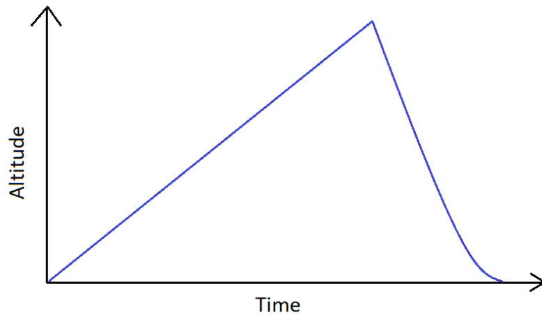
Figure 7: Example Flight Profile of Expanding Volume Balloon
