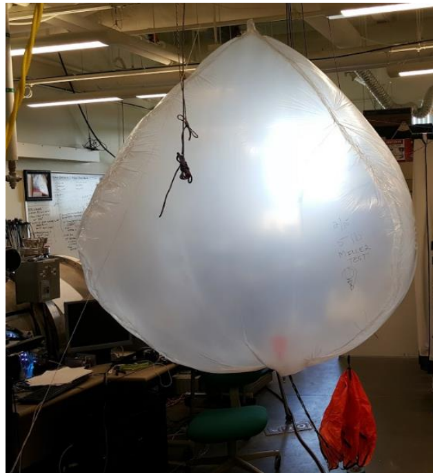
Figure 28: Leak Checking of ZP Balloon
