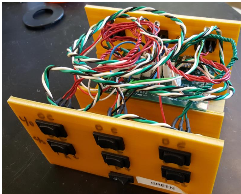
Figure 16: Remote for Tethered Sampler Boxes
