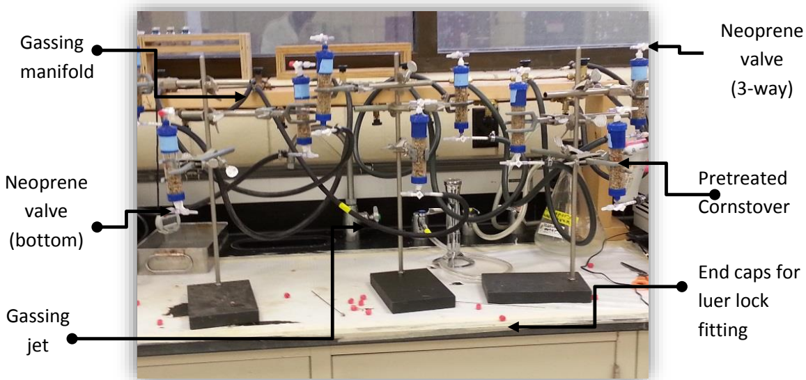
Figure 17: Flushing columns loaded with cornstover
