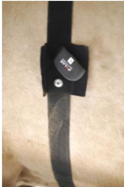
Figure 3-9 Snapping mechanism for attaching the Wearlink® transmitter to the strap.
