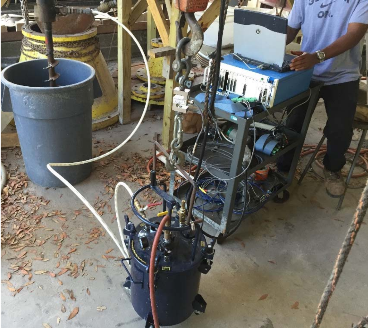
Figure 4.10 Grout calibration setup.
