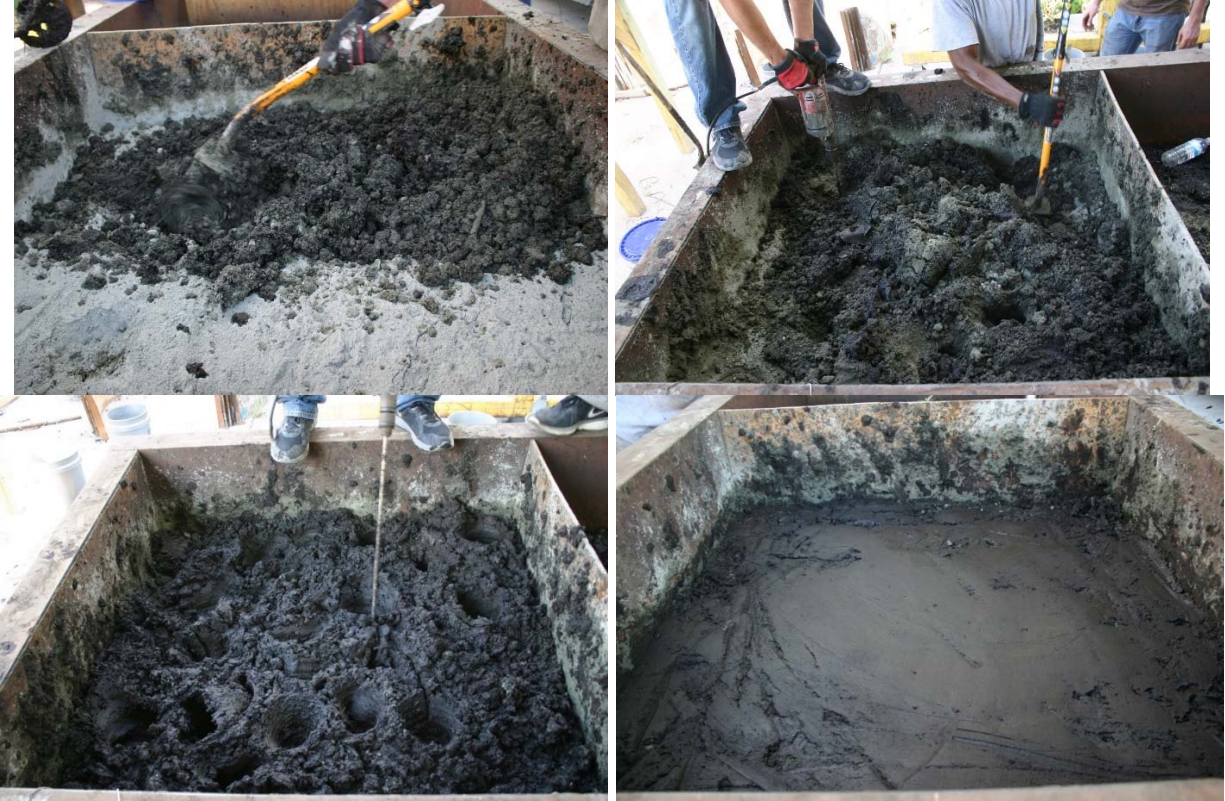
Figure 4.31 Dry mixing progression, part 2 of 2.
