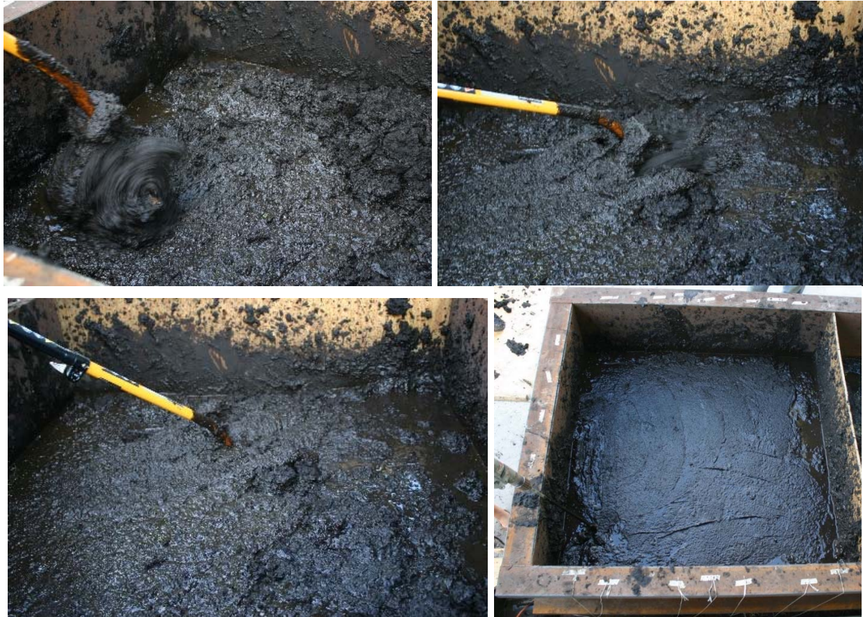
Figure 4.28 Tiller in soil prior to cement introduction.
