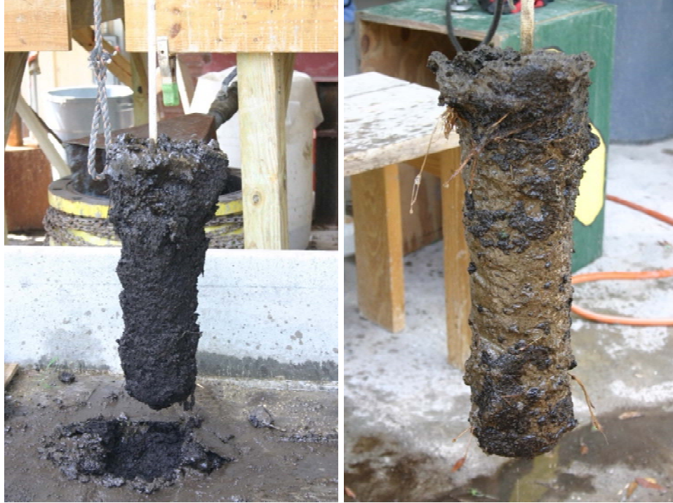
Figure 4.18 Wet mixed column (left) and after washed (right).
