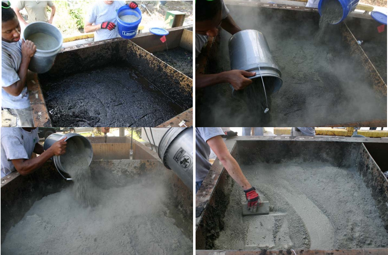
Figure 4.29 Introducing dry cement to soil.
