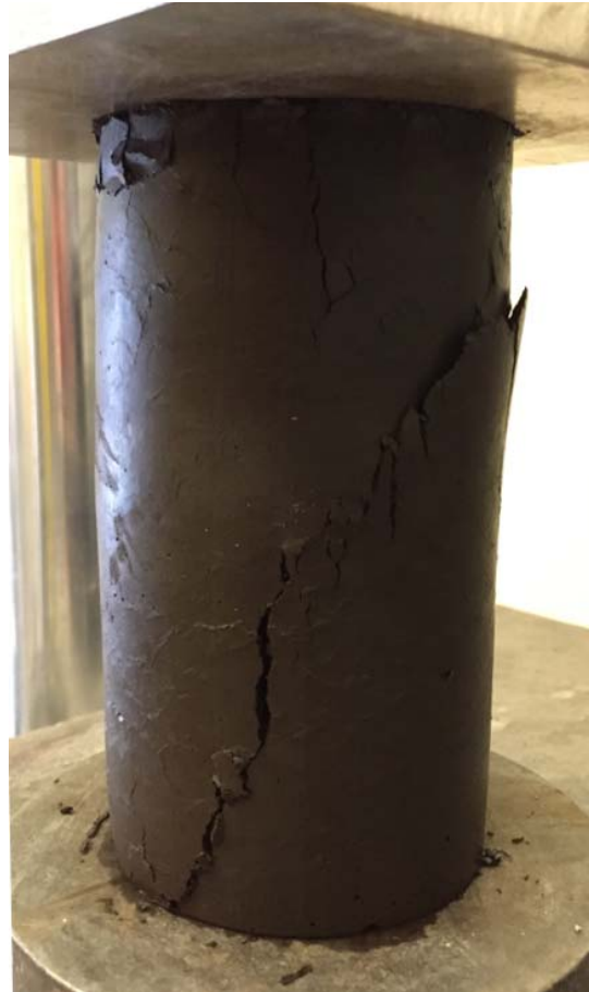
Figure 3.7 Unconfined compression testing of 3 x 6 in. cylinders.
