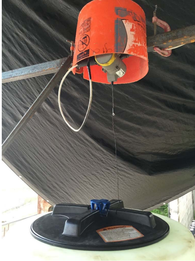
Figure 4.35 String line transducer mounted above water tank.
