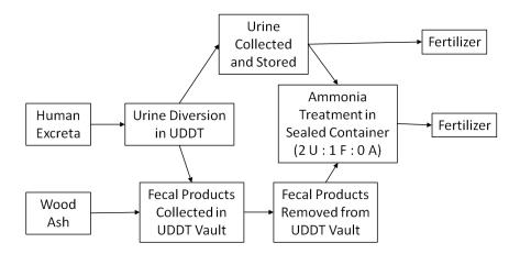
Figure 14: Recommended ammonia treatment process diagram
