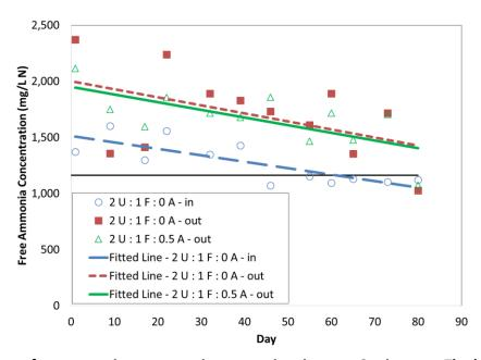
Figure 11: Average free ammonia concentrations over time in stage 3 mixtures. The horizontal black line represents the concentration required to achieve 2-log<sub>10</sub> inactivation of *Ascaris* eggs in 60 days at a temperature of 23°C (Fidjeland et al., 2013).
