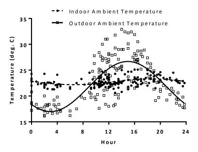
Figure 12: Ambient temperature measurements with "typical day" models over 24-hour period
