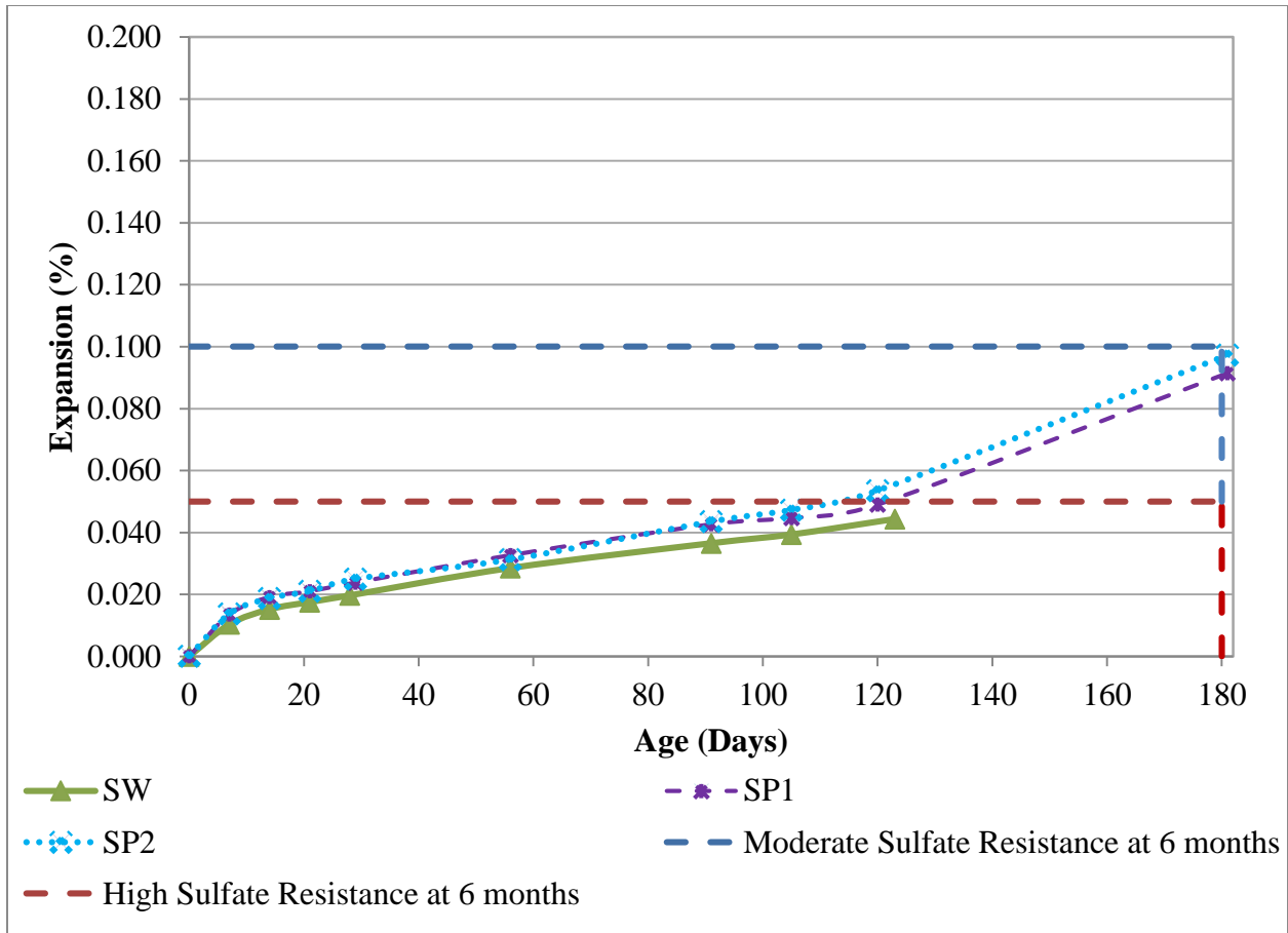
Figure 51: Effect of SP on Length Change of Mortar Sample in 5% Na 2 SO 4 Solution
