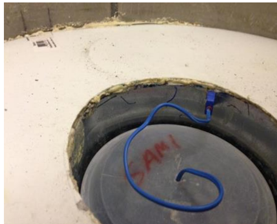
Figure 7: Middle Thermocouple Placed and Plugged In
