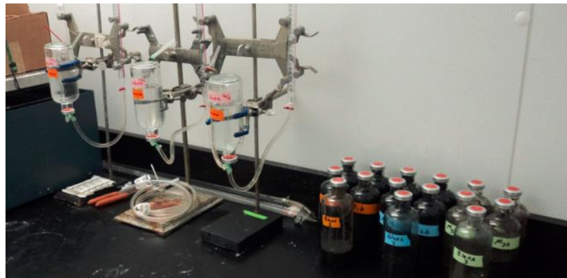
Figure E.2: Bench-scale experiment 1 setup, including methane measuring apparatus.
