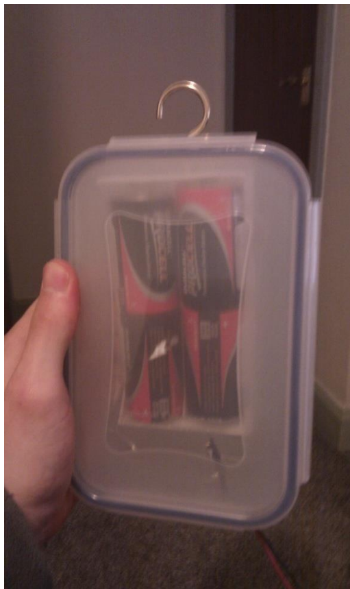
Figure 31. Water resistant battery pack container. A hole is cut in the bottom to allow the LED attachment to clip to the battery pack.
