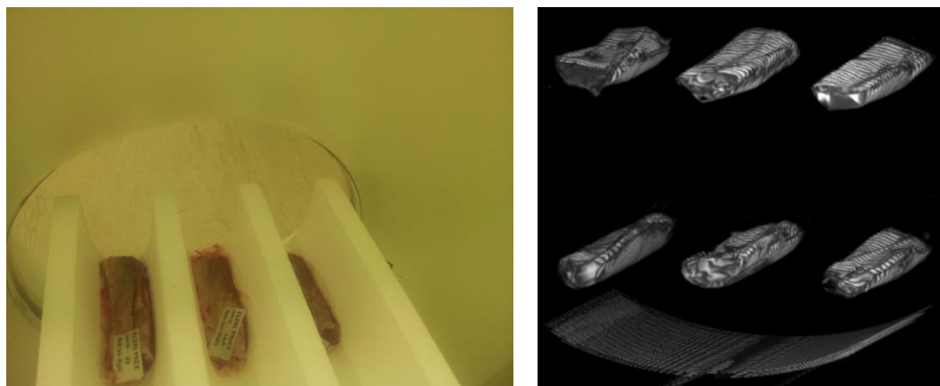
Figure i: Dissected loins orientated and positioned in the multiplex frame (left), 3D rendered image of multiplex scanning (right)
