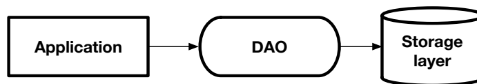
Figure 2.2: The DAO layer is located between the application and the storage layer. The DAO layer isolates the application logic from persistence domain and allows them to evolve independently providing them with a reference interface.
