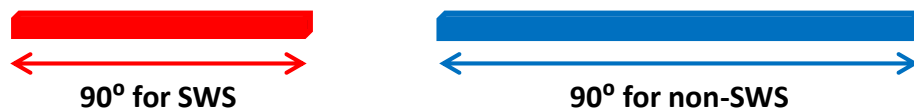
Figure: 2.1 Comparison of the physical length of a regular structure and slow wave structure for the same electrical length.
