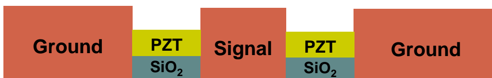
Figure 4.4: Growth of PZT on non-conducting SiO 2 for coplanar devices.
