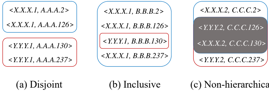
Figure 3.2: The relationship between the sets of the addresses grouped by last-hop routers. \langle X, Y \rangle denotes X is a last-hop router of a destination Y .
