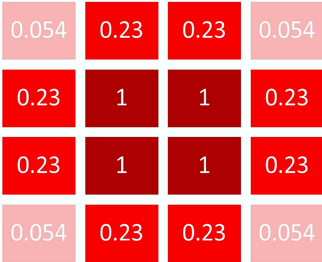
Fig. 5.5: Synthesized taper excitation coefficient for SLL of 25 dB.
