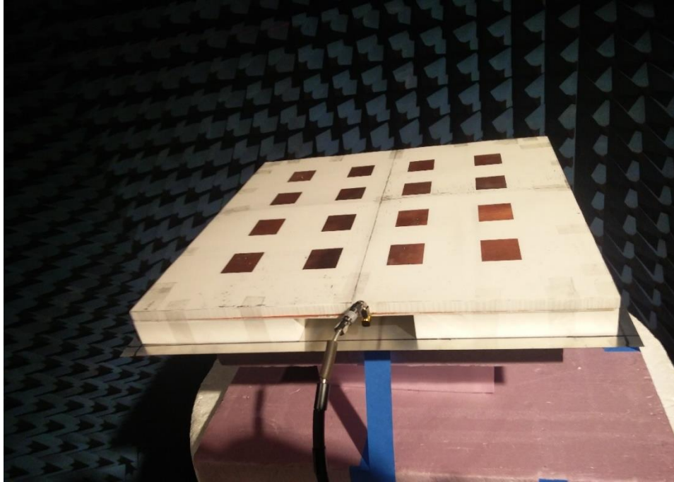
Fig. 6.9: Radiation pattern measurement setup for array with reflector.
