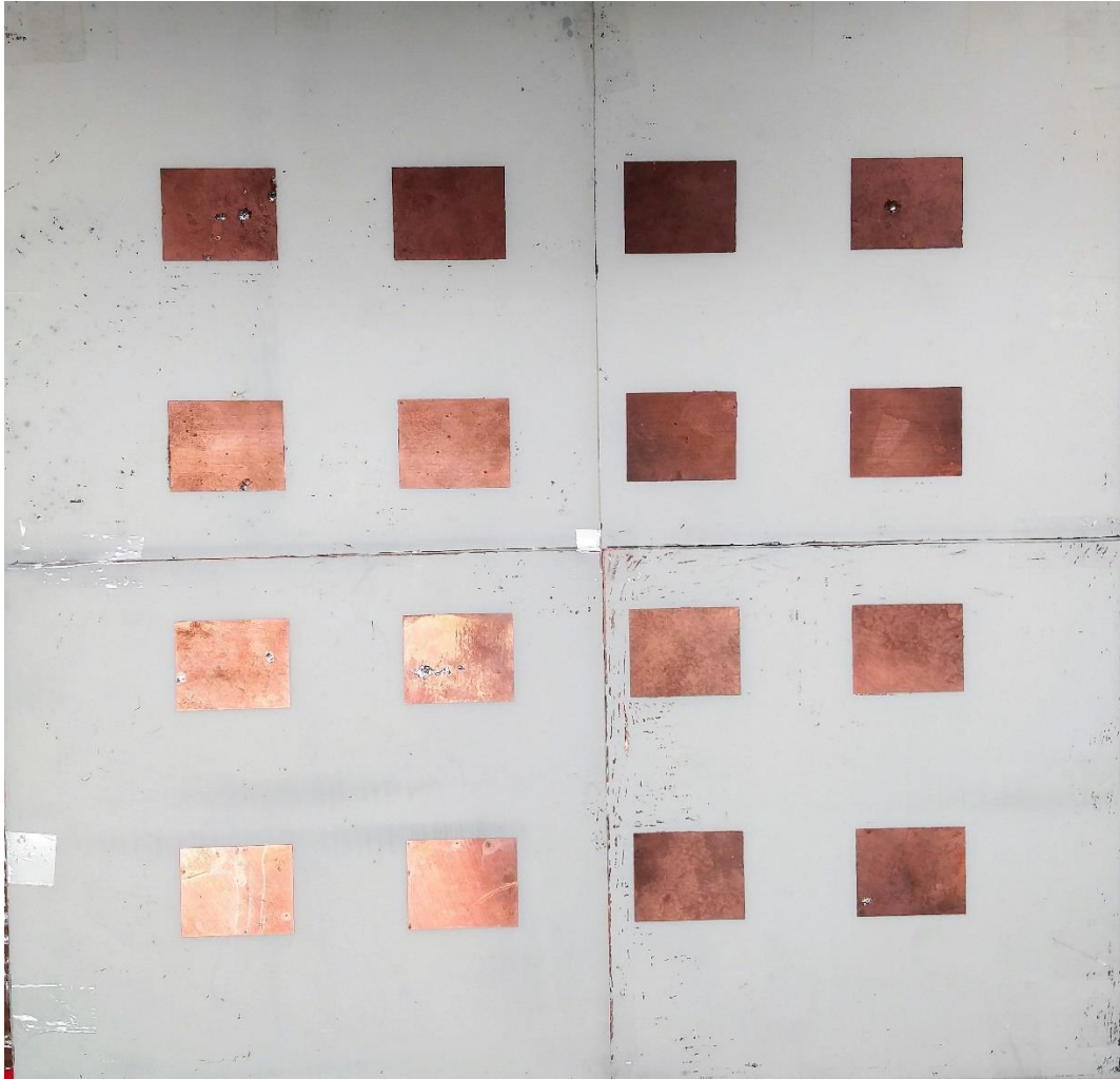
Fig. 6.1: Top view of array.
