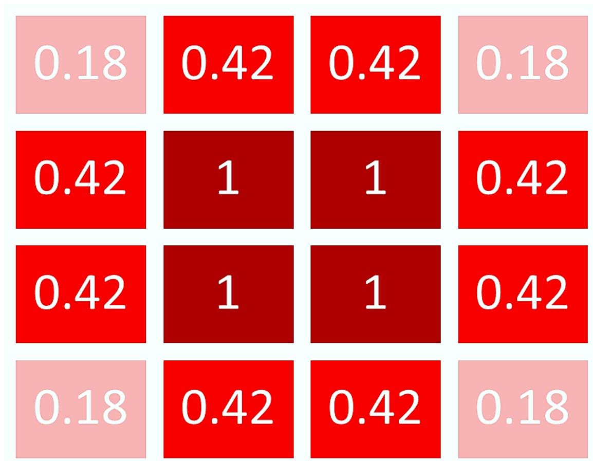
Fig. 5.3: Dolph-Chebyshev taper excitation coefficient.
