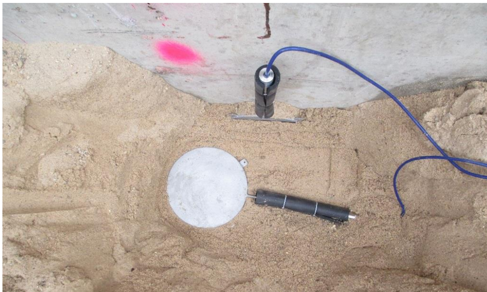
Figure 140. Sensor installation behind Badger Road Bridge
