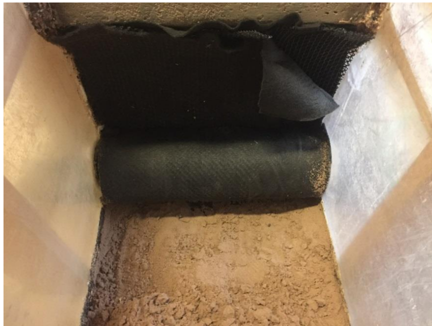
Figure 73. Geocomposite wrapped drain tile (top view)
