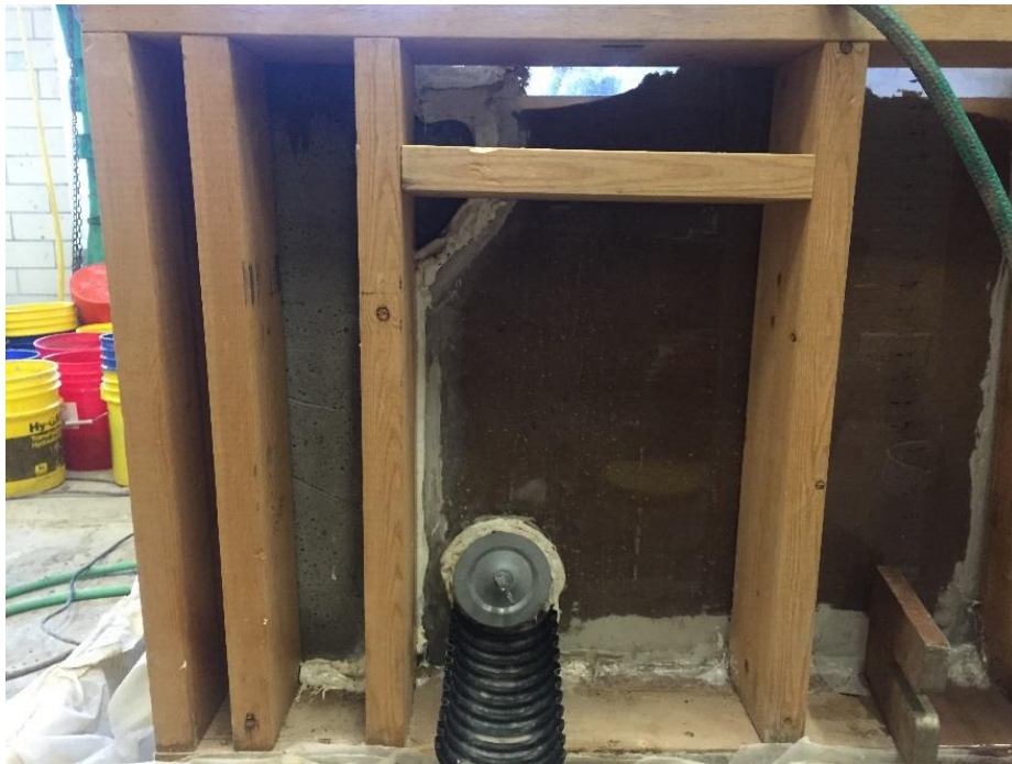
Figure 33. Drain tile plugged for saturation
