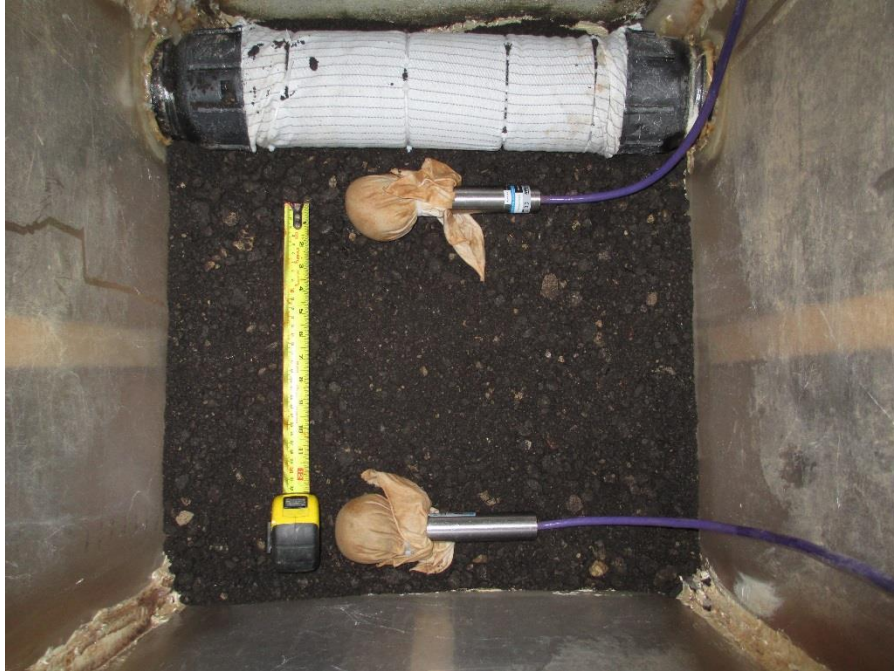
Figure 43. Geokon 3400 dynamic piezometers inside abutment model
