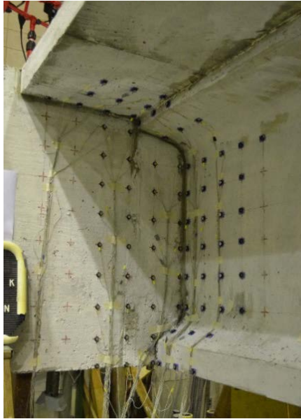
Figure 3.34: LED configuration at connection region
