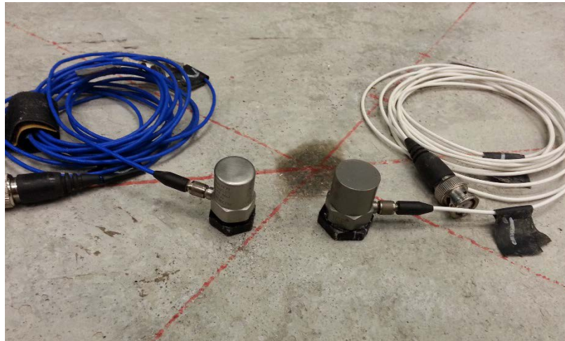
Figure 2.1. PCB model 621B51 (left) and 353B33 (right) piezoelectric accelerometers used in this study.
