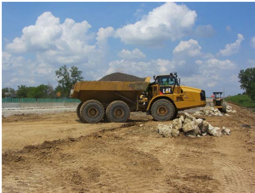
Figure 29. Caterpillar 740B dump truck used to place loose fill materials
