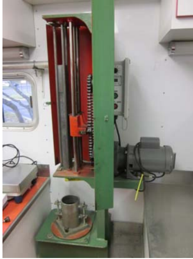
Figure 15. Mechanical Proctor setup
