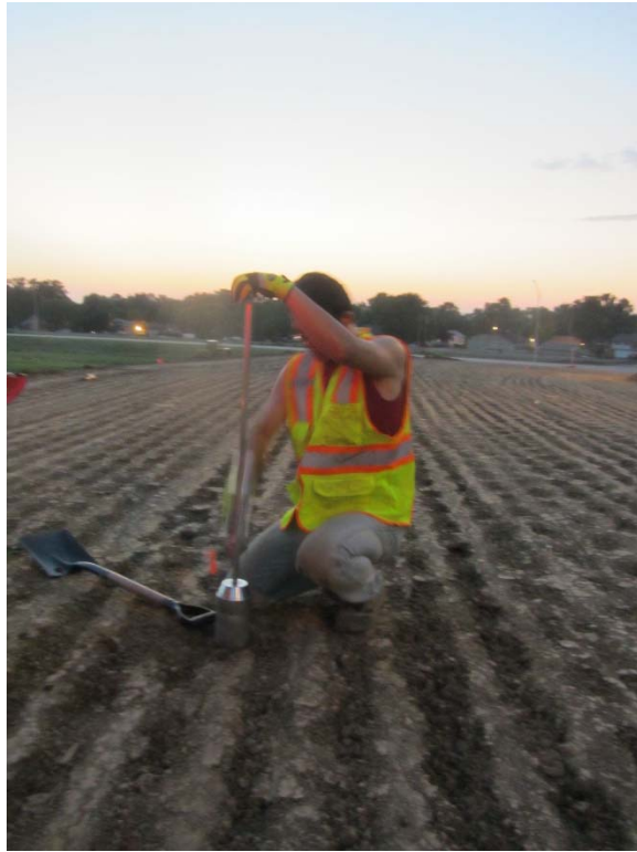
Figure 90. ISU in situ drive cylinder test
