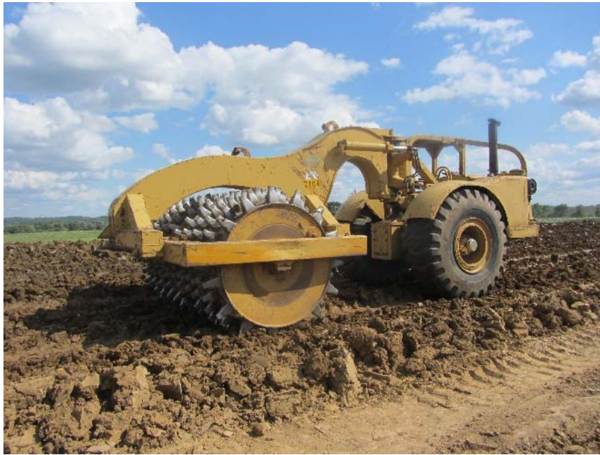
Figure 56. Sheepfoot roller used for soil compaction
