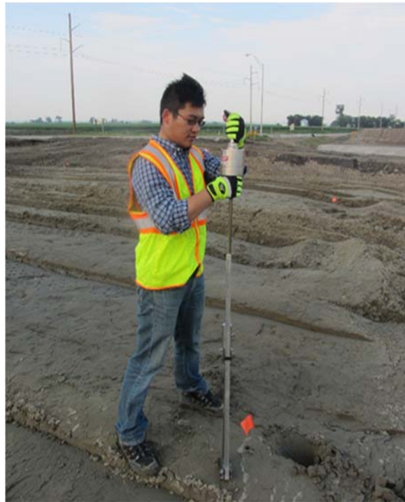
Figure 100. ISU DCP testing
