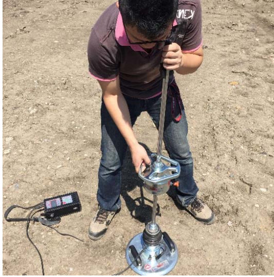
Figure 10. Light weight deflectometer test
