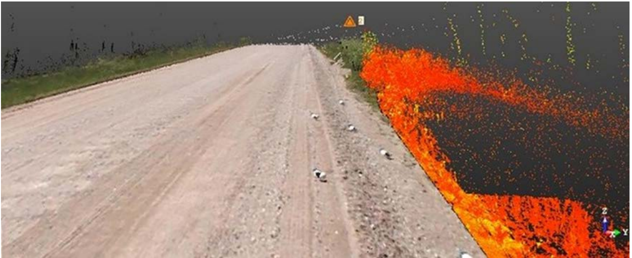
Figure 18. Registered point cloud for data acquired from two stations.
