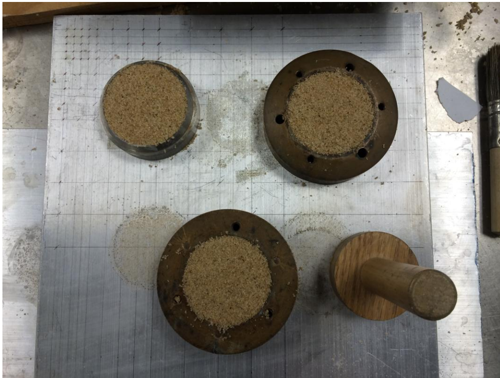
Figure 16. Preparation method for the polymer-stabilized sand specimens.
