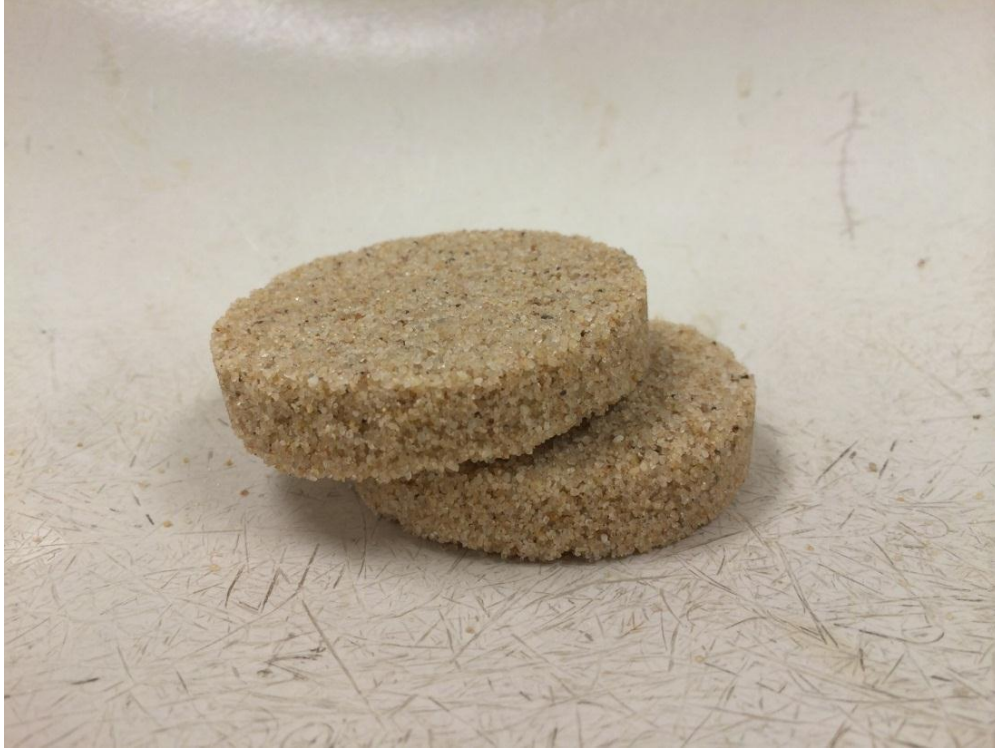
Figure 33. 2% polymer-amended sand specimen after failure.
