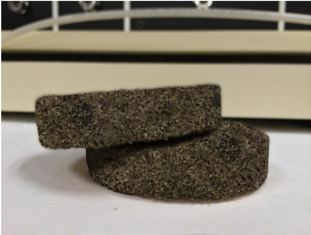
Figure 32. 8% cement-amended sand specimen after failure.
