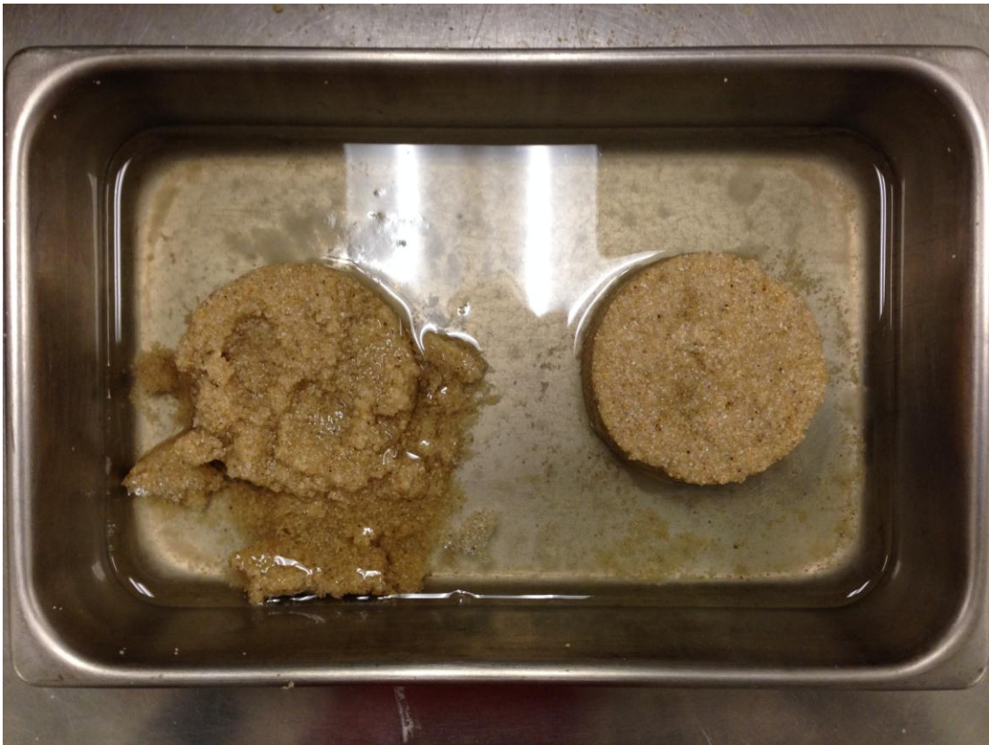
Figure 80. Submerged polymer-amended specimens. The specimen on the left was gently probed with a spatula.
