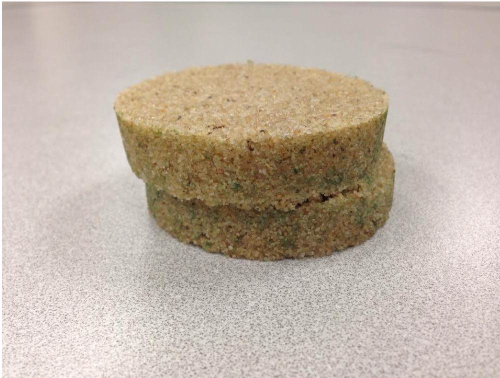
Figure 34. 4% polymer-amended sand specimen after failure.
