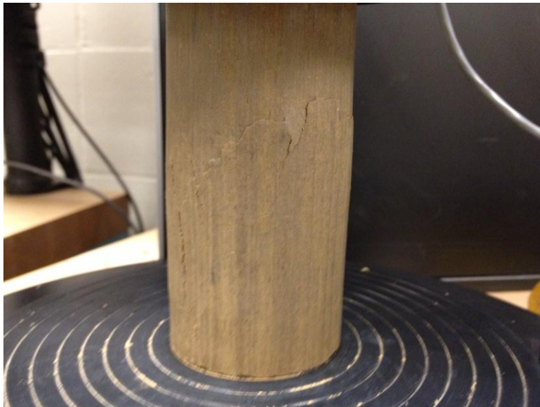
Figure 22. Typical failure of monomer-treated specimens in unconfined compression tests.
