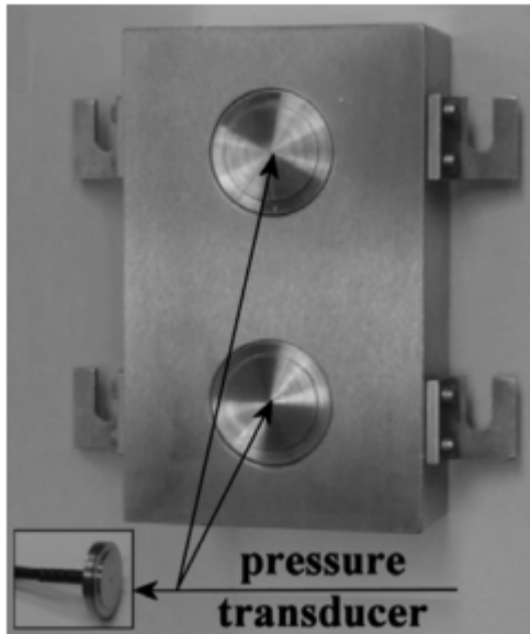
Figure 6-3. Lateral loading plate used to measure out of plane stress (after Wanatowski 2005)
